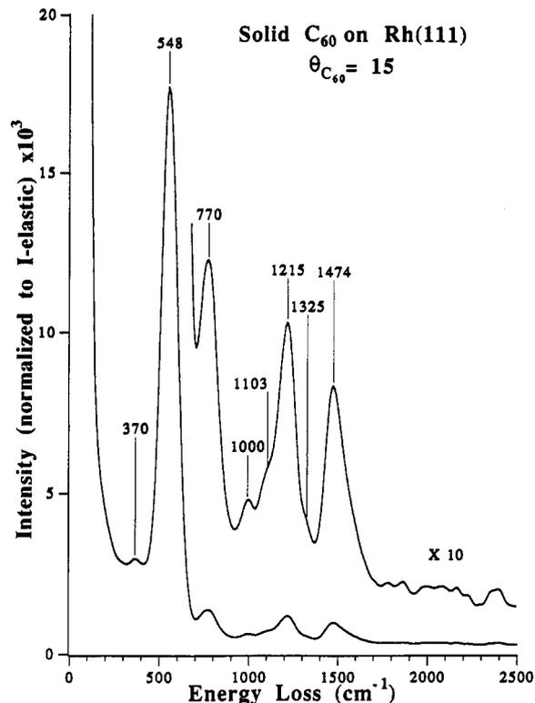
**Figure 3.** HREELS spectrum from a  $C_{60}$  multilayer film ( $\theta_{C_{60}} = 15$ ) on Rh(111).
