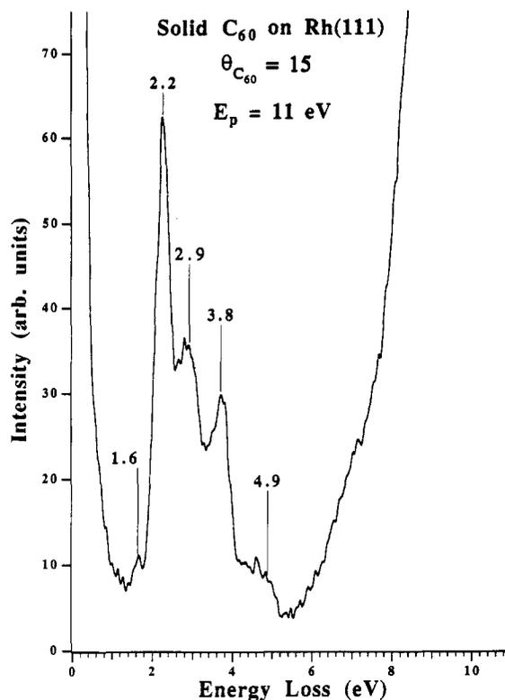
Figure 7. ELS spectrum at  $E_p = 11$  eV from a  $C_{60}$  multilayer film ( $\theta_{C_{60}} = 15$ ) on Rh(111).
