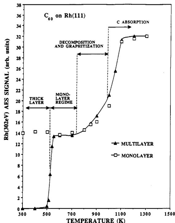
**Figure 2.** Rh(302 eV) AES signal as a function of annealing temperature for multilayer ( $\theta_{C_{60}} = 15$ ) and monolayer ( $\theta_{C_{60}} = 1$ )  $C_{60}$  films on Rh(111).
