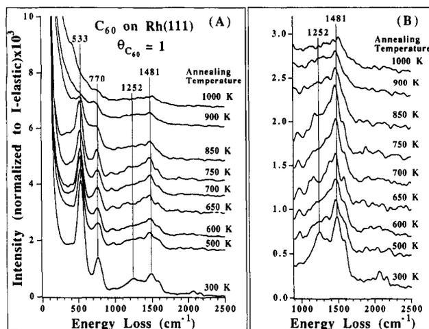
Figure 5. HREELS spectra from a monolayer C<sub>60</sub> film on Rh(111) annealed to increasing temperatures.
