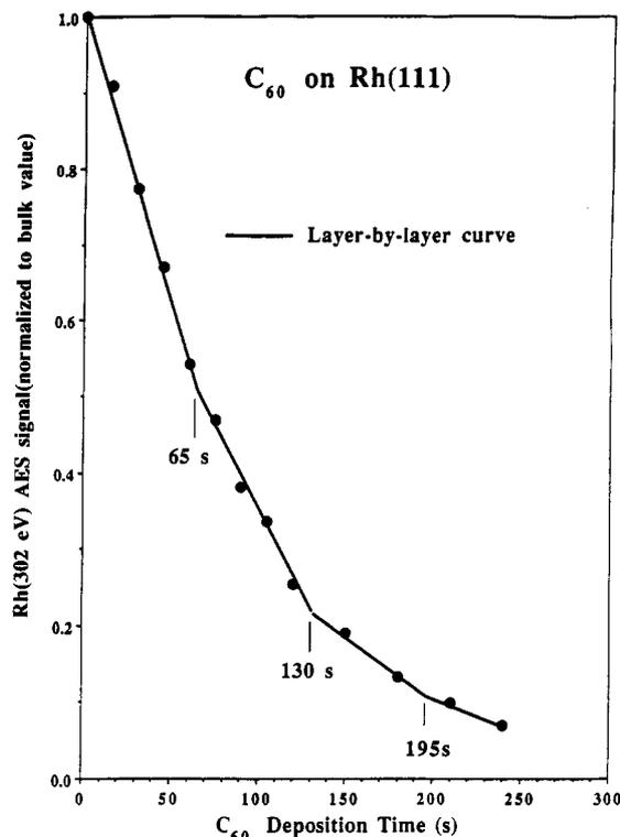
Figure 1. Rh(302 eV) AES signal versus C<sub>60</sub> deposition time monitoring the vapor deposition of C<sub>60</sub> on Rh(111) at room temperature.
