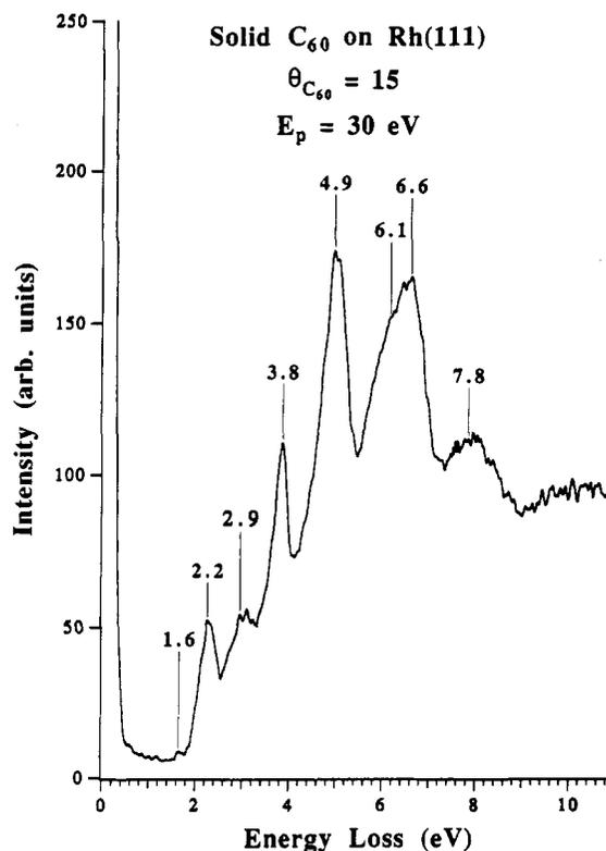
Figure 8. ELS spectrum at  $E_p = 30$  eV from a  $C_{60}$  multilayer film ( $\theta_{C_{60}} = 15$ ) on Rh(111).
