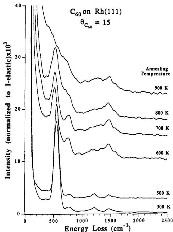
Figure 6. HREELS spectra from a  $C_{60}$  multilayer film ( $\theta_{C_{60}} = 15$ ) on Rh(111) annealed to increasing temperatures.
