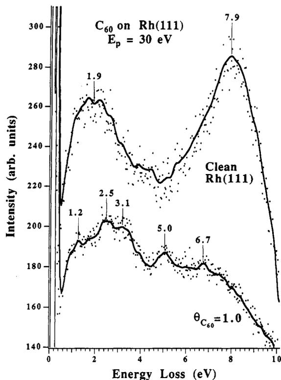
**Figure 9.** ELS spectra at  $E_p = 30$  eV from a clean Rh(111) surface and a C<sub>60</sub> monolayer on Rh(111). A solid curve obtained by smoothing the measured data is shown in addition to the measured data points in order to discern the spectral features.
