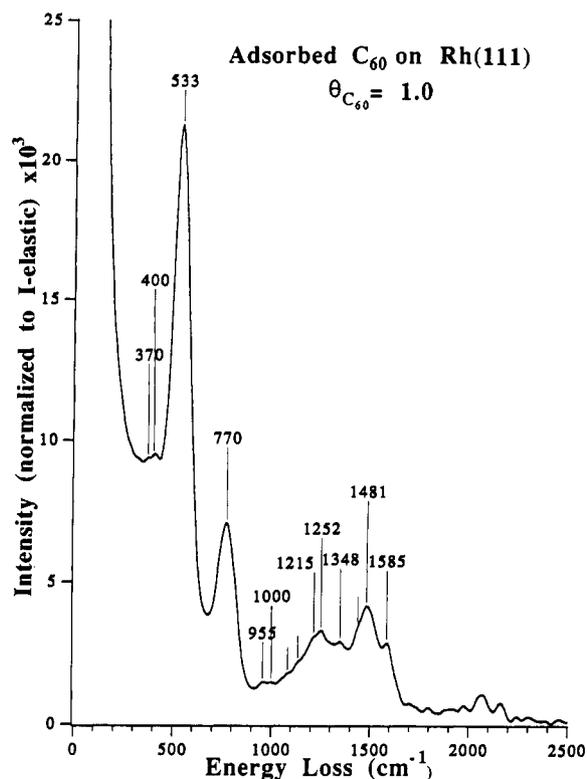
Figure 4. HREELS spectrum from a monolayer C<sub>60</sub> film on Rh(111).
