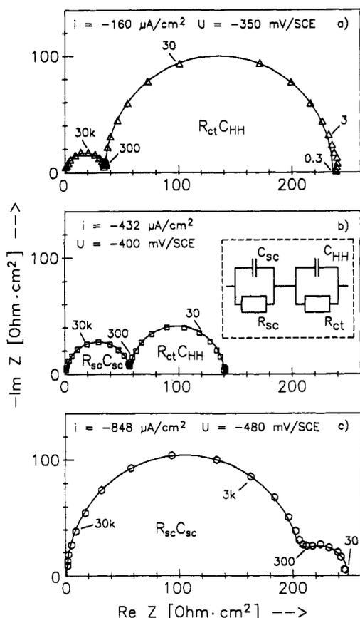
**Figure 4.** Impedance data for p-InP in 1 M H<sub>2</sub>SO<sub>4</sub> (N<sub>2</sub>) at a constant illumination intensity ( $i_{ph} \approx -1.0$  mA/cm<sup>2</sup>) and varying current densities  $i$ . Measurement points and fitted curves; the fitting parameters to the circuit in the insert are listed in Table I.
