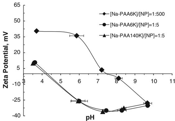
**Fig. 3** The effect of PAA and pH on the zeta potential of 2-line ferrihydrite particles at a solid content of 50 mg/L and sodium strength of 10 mM. The vertical error bars are smaller than the data point symbols
