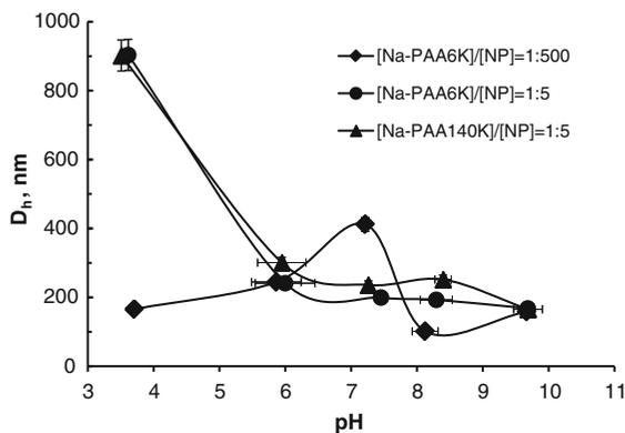
**Fig. 4** The effect of PAA and pH on the hydrodynamic diameter of 2-line ferrihydrite particles at a solid content of 50 mg/L and sodium strength of 10 mM
