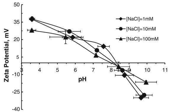
**Fig. 1** The effect of background electrolyte and pH on the zeta potential of 2-line ferrihydrite particles at a solid content of 50 mg/L
