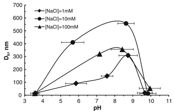
**Fig. 2** The effect of background electrolyte and pH on the hydrodynamic diameter of 2-line ferrihydrite particles at a solid content of 50 mg/L. The vertical error bars are smaller than the data point symbols
