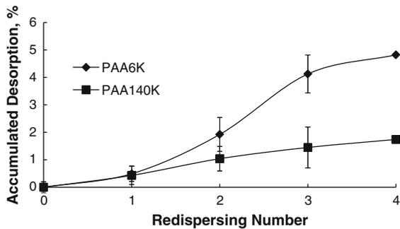
**Fig. 7** Polymer desorption measurements using multiple redispersions in 100 mM NaCl for polymer coatings added after the NP synthesis. The initial particle, prior to any desorption is plotted on the origin. Each vertical error bar represents an accumulation of errors from previous samples
