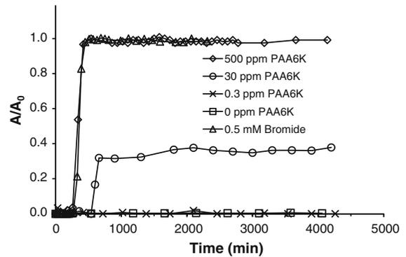
**Fig. 8** Transport measurements through natural quartz and columns showing breakthrough curves of 2-line ferrihydrite nanoparticles that have been coated by PAA6K using various polymer solution concentrations. The bromide breakthrough curve provides a reference for a solute that is not interacting with the solid matrix. The nanoparticle feed solution was controlled to be pH = 6.5
