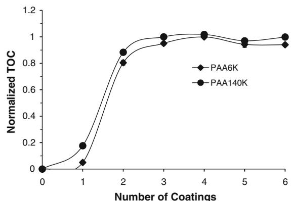
**Fig. 6** A normalized total organic carbon (TOC) value in the supernatant solution was measured after each repeated coating/centrifuging step to track the extent of polymer adsorption on previously prepared nanoparticles
