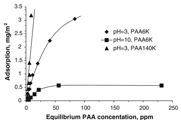
**Fig. 5** Adsorption isotherms of PAA on 2-line ferrihydrite nanoparticles for two molecular weights of the polymer and two values of pH. [NaCl] = 10 mM, [2-line ferrihydrite] = 2.25 g/L, and the other two solid curves are the fittings to the experimental data
