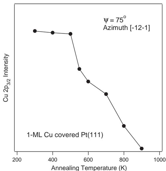
**Fig. 2.** Cu  $2p_{3/2}$  XPS intensity for a 1-ML Cu film deposited on Pt(111) after annealing to several temperatures. The decrease in the Cu  $2p_{3/2}$  intensity above 500 K indicates that alloying takes place at these high temperatures. Annealing at 900 K nearly eliminated the Cu signal, implying that Cu migrates deeply into the crystal.
