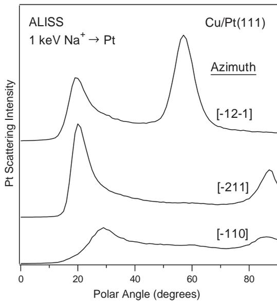
Fig. 6. Polar angle scans for 1-keV  $\text{Na}^+$  ions scattered from Pt atoms for the Cu/Pt(111) alloy along the [-12-1], [-211], and [-110] azimuthal directions, respectively.
