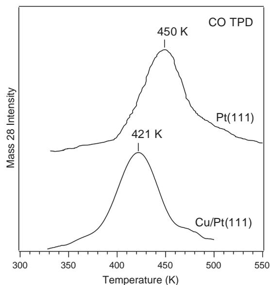
**Fig. 9.** CO TPD spectra from clean Pt(111) and the Cu/Pt(111) alloy surface after a 0.05 L CO exposure at room temperature.
