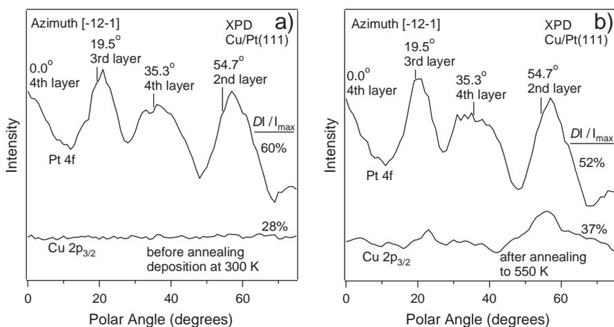
**Fig. 4.** (a) XPD polar scans along the  $[-12-1]$  azimuth for 1-ML Cu deposited on Pt(111) at 300 K before annealing. (b) XPD polar scans along the  $[-12-1]$  azimuth for 1-ML Cu deposited on Pt(111) at 300 K after annealing at 550 K and forming a Cu–Pt alloy. Angle labels above the curves are predicted enhancement directions based on the known structure of Pt(111).
