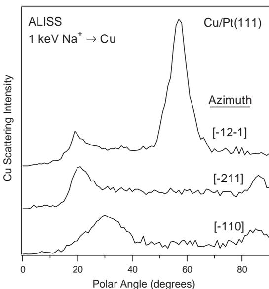
Fig. 7. Polar angle scans for 1-keV  $\text{Na}^+$  ions scattered from Cu atoms for the Cu/Pt(111) alloy along three different directions, the long azimuths [-12-1], [-211], and the short azimuth [-110]. The observed enhanced scattering features contain contributions from 1<sup>st</sup>, 2<sup>nd</sup>, and 3<sup>rd</sup>-layer Cu atoms.
