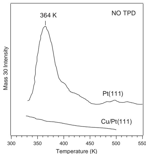
**Fig. 10.** NO TPD spectra from clean Pt(111) and the Cu/Pt(111) alloy surface after a 3 L NO exposure at room temperature.
