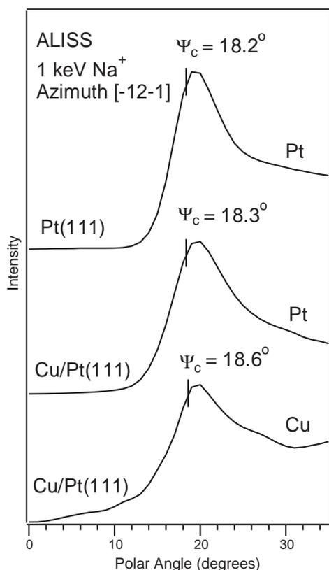
**Fig. 8.** Polar scans of first-layer scattering features for Pt (from clean Pt(111) and the Cu/Pt(111) alloy) and Cu (from the Cu/Pt(111) alloy) along the [-12-1] azimuthal direction. The position of each critical angle  $\Psi_c$  is marked by a short bar.
