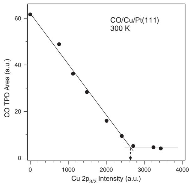
**Fig. 1.** Determination of the Cu monolayer coverage based on an evaluation of the CO TPD area as a function of the Cu 2p $_{3/2}$  XPS intensity for Cu deposited on Pt(111) at 300 K. The arrow denotes 1-ML Cu.
