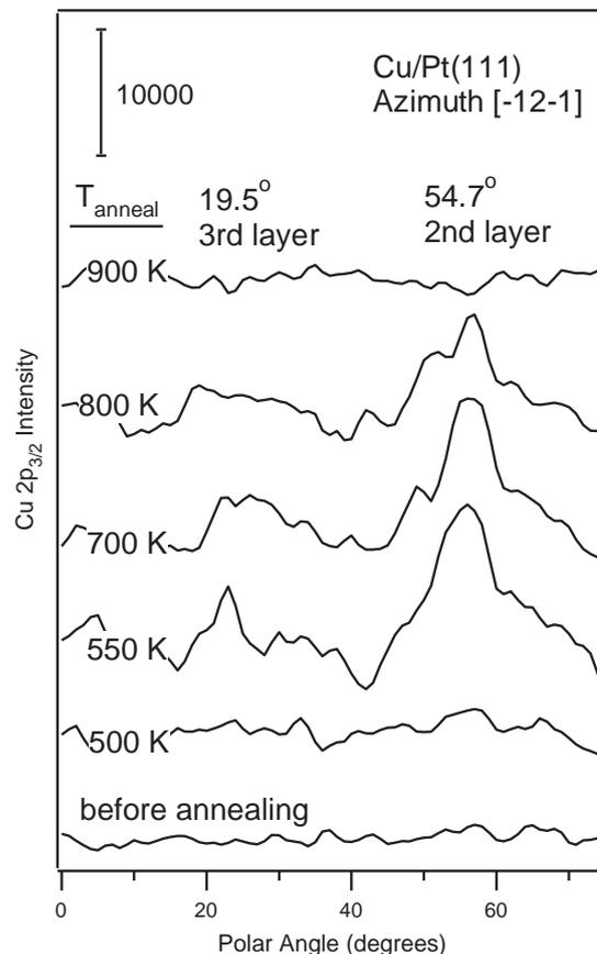
**Fig. 3.** XPD polar scans of the Cu  $2p_{3/2}$  intensity of 1-ML Cu deposited on Pt(111) over polar angles of  $\psi = 0^\circ$  to  $75^\circ$  along the  $[-12-1]$  azimuthal direction after annealing. The enhanced Cu  $2p_{3/2}$  diffraction features were observed after annealing at 550 K, indicating that alloying occurs at this temperature. Angle labels above the curves are predicted enhancement directions based on the known structure of Pt(111).
