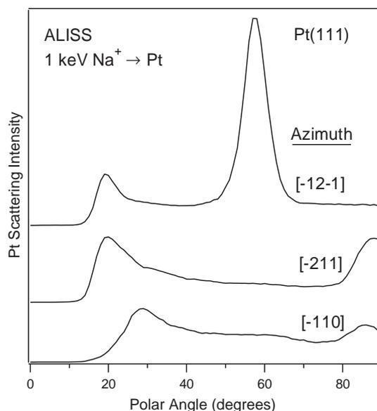
**Fig. 5.** Polar angle scans for 1-keV  $\text{Na}^+$  ions scattered from the clean Pt(111) surface along the  $[-12-1]$ ,  $[-211]$ , and  $[-110]$  azimuthal directions, respectively.
