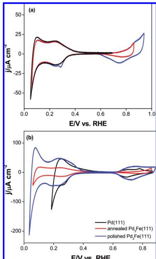
**Figure 2.** (a) Voltammetry curves for an annealed Pd<sub>3</sub>Fe(111) in 0.1 M HClO<sub>4</sub> solution with different positive potential windows. (b) Voltammetry curves for an annealed (red line) and a polished Pd<sub>3</sub>Fe(111) (blue line), and Pd(111) (black line) in 0.1 M HClO<sub>4</sub> solution. Scan rate: 20 mV s<sup>-1</sup>.
