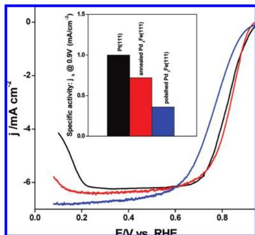
**Figure 4.** Polarization curves for the ORR on the annealed (red) and polished (blue) Pd<sub>3</sub>Fe(111) surfaces and also on a Pt(111) surface at 1600 rpm in oxygen-saturated 0.1 M HClO<sub>4</sub> at room temperature; scan rate: 20 mV s<sup>-1</sup>. Inset shows the bar plot for the comparison of ORR specific surface activities of the corresponding three surfaces at 0.9 V<sub>RHE</sub>.
