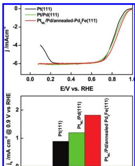
**Figure 7.** (a) Polarization curves for the ORR on a Pt monolayer covered annealed-Pd<sub>3</sub>Fe(111) (red), annealed-Pd(111) (green), and Pt(111) surfaces (black) at 1600 rpm in oxygen-saturated 0.1 M HClO<sub>4</sub> at room temperature; scan rate: 20 mV s<sup>-1</sup>. Inset shows the bar plot for the comparison of ORR specific activities of the corresponding three surfaces at 0.9 V<sub>RHE</sub>.
