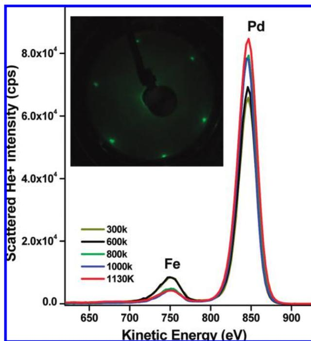
**Figure 1.** LEIS spectra (1 keV He<sup>+</sup>) for a Pd<sub>3</sub>Fe(111) surface annealed to various temperatures. Inset shows a (1 × 1) LEED pattern for a Pd<sub>3</sub>Fe(111) surface annealed to 1200 K. The electron beam energy was 55 eV.
