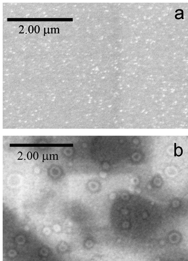
**Fig. 8.** SEM images of the 10-nm thick sputtered Au film before (a) and after ECRBS Au dissolution experiment (b). The Au film is initially fairly homogeneous, but after the dissolution experiments, shows altered Au regions with a diameter of  $\sim 300 \text{ nm}$  that arise from radiolysis and/or Au dissolution.
