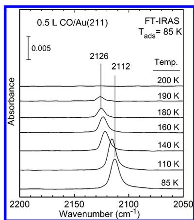
**Figure 5.** Companion IRAS spectra to Figure 3 that were obtained after dosing 0.5 langmuir CO on Au(211) at 85 K and then subsequently flashing the crystal to various temperatures in the range of 85–200 K. The spectra were taken after recooling the surface to 85 K. The  $\nu_{\text{CO}}$  band appeared at 2112  $\text{cm}^{-1}$  at 85 K and shifted to 2126  $\text{cm}^{-1}$  after flashing to 190 K. Flashing above 200 K removes all CO from the surface.
