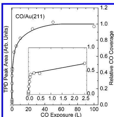
**Figure 2.** Uptake curve for CO adsorption on Au(211) at 85 K. This was constructed from the CO TPD peak areas from data presented in Figure 1. The inset shows CO uptake in the low-exposure regime (0–2.5 langmuir) on an expanded scale. CO adsorbs more efficiently below 0.1 langmuir exposure, and then the CO sticking coefficient decreases significantly.
