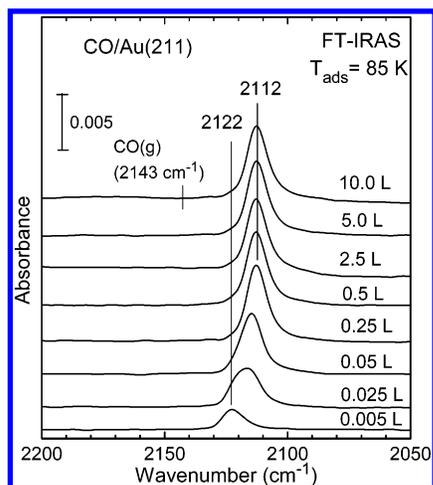
**Figure 4.** Vibrational spectra from IRAS obtained after dosing 0.005–10 langmuir CO on Au(211) at 85 K. The  $\nu_{\text{CO}}$  mode of CO adsorbed on Au(211) after the lowest exposure (0.005 langmuir) occurs at 2122  $\text{cm}^{-1}$ , and then it shifts to 2112  $\text{cm}^{-1}$  with increasing exposure. The position of  $\nu_{\text{CO}}$  (2143  $\text{cm}^{-1}$ ) for gas-phase CO is marked on the top spectrum for comparison.
