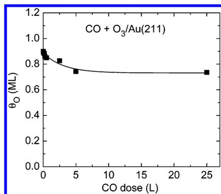
**Figure 7.** Plot of the coverage of oxygen left at the Au(211) surface following the CO exposures reported in Figure 6 and heating during subsequent TPD. The oxygen coverage was determined by the O<sub>2</sub> TPD peak areas obtained simultaneously in these experiments. The amount of oxygen at the Au(211) surface at 85 K was initially reduced efficiently by small CO doses, indicating a fast CO oxidation reaction transient, but then some oxygen that is much less reactive remains on the surface.
