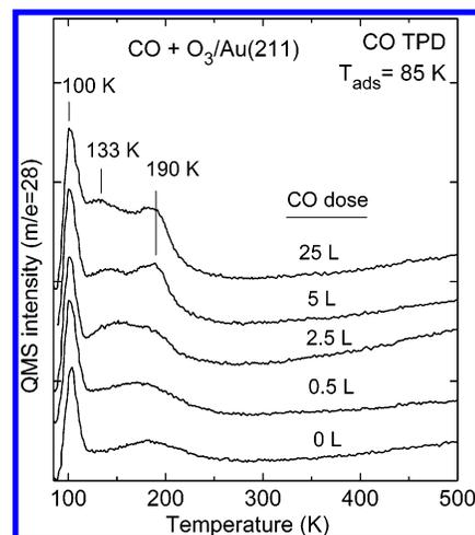
**Figure 6.** CO TPD curves obtained after exposing CO on an oxygen-precovered surface produced by a 100 langmuir  $\text{O}_3$  exposure on the Au(211) surface at 85 K to create a saturation coverage of O adatoms. CO TPD peaks at 133 and 190 K indicate that some CO is reversibly adsorbed on the Au(211) after large CO doses.
