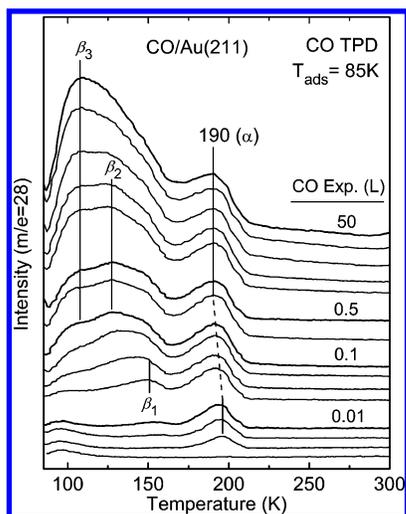
**Figure 1.** CO TPD curves obtained after dosing 0.0025–50 langmuir (L) CO on Au(211) at 85 K. Results are shown for CO exposures of 0, 0.0025, 0.005, 0.01, 0.025, 0.05, 0.1, 0.25, 0.5, 1, 2.5, 5, 10, 25, and 50 langmuir. Peaks are identified as  $\alpha = 190$  K,  $\beta_1 = 150$  K,  $\beta_2 = 127$  K, and  $\beta_3 = 109$  K. The bottom curve is for CO desorption from background accumulation only, with no CO dose given.
