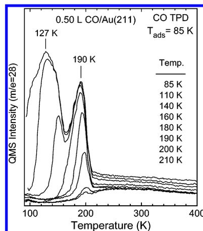
**Figure 3.** CO TPD curves obtained after dosing 0.5 langmuir (L) CO on Au(211) at 85 K and then preannealing to various temperatures. CO remains only at the Au(211) step sites after annealing to 160 K.
