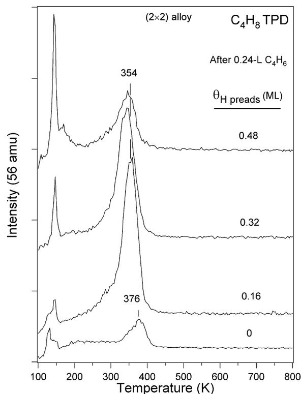
Fig. 2. Butene,  $C_4H_8$  TPD spectra after after 0.24-L 1,3-Butadiene exposures on the clean and H-precovered  $(2 \times 2)$ Sn/Pt(111) alloy at 100 K.
