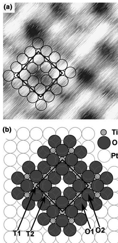
Fig. 13. (a) STM topograph from a titanium-oxide film on Pt(100) exhibiting a  $(2\sqrt{2} \times 2\sqrt{2})R45^\circ$  structure. (b) Tentative model of the  $(2\sqrt{2} \times 2\sqrt{2})R45^\circ$  structure. The superimposed black squares indicate the  $(2\sqrt{2} \times 2\sqrt{2})R45^\circ$  unit cell. This structure presents two different environments for Ti atoms ( $T1$  and  $T2$ ) and O atoms ( $O1$  and  $O2$ ).
