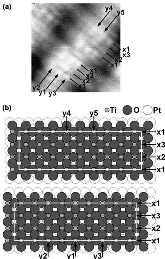
Fig. 12. (a) STM topograph from a titanium-oxide film on Pt(100) exhibiting a  $(4 \times 13)$  structure. (b) Tentative model of the  $(4 \times 13)$  structure. The superimposed white rectangle indicates the  $(4 \times 13)$  unit cell. The rows  $x1-5$  and  $y1-3$  correspond to each other in each figure.
