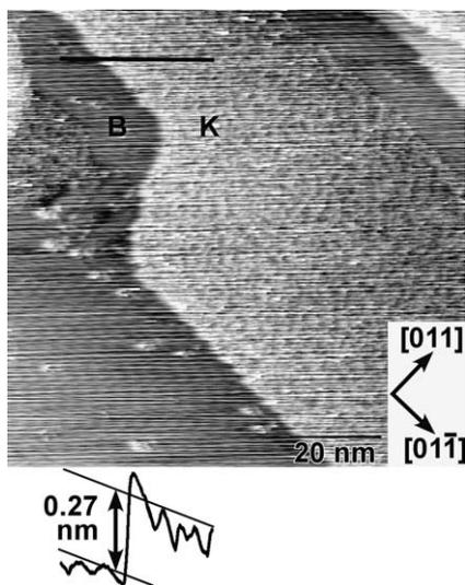
Fig. 7. STM topograph of the  $(3 \times 5)$  oxide film on Pt(100) after further oxidation using 3-L  $O_3$  with the substrate at 600 K ( $V_s = 1$  V,  $I_t = 0.16$  nA). Domains B and K are assigned to the  $(3 \times 5)$  oxide film and more deeply oxidized regions, respectively. The cross-section of the line scan indicated in the image is shown directly below.
