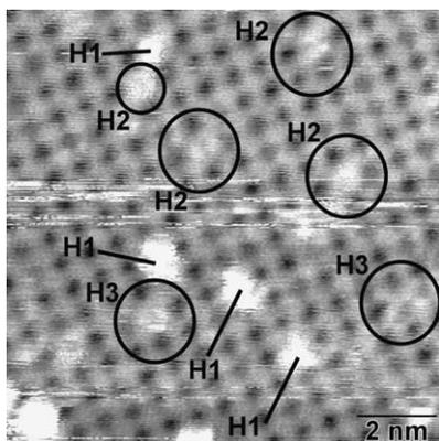
Fig. 5. STM topograph showing defect sites on a titanium-oxide film on Pt(100) exhibiting a  $(2\sqrt{2} \times 2\sqrt{2})R45^\circ$  structure ( $V_s = 0.39$  V,  $I_t = 0.87$  nA). We attribute the defects labeled *H1*–*H3* as due to population of a second layer, Ti atoms in the center of the unit cell, and rotated  $(2\sqrt{2} \times 2\sqrt{2})R45^\circ$  nets, respectively.
