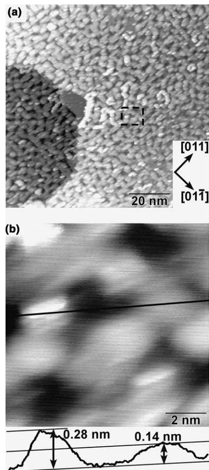
Fig. 9. STM topographs of the  $(3 \times 5)$  oxide film on Pt(100) after further oxidation using 15-L  $O_3$  with the substrate at 600 K. (a) Titania clusters ( $V_s = 1.1$  V,  $I_t = 0.78$  nA). (b) Expanded view of the region indicated by the superimposed dashed box in (a) ( $V_s = 0.2$  V,  $I_t = 0.74$  nA). The cross-section of the line scan indicated in the image is shown directly below.
