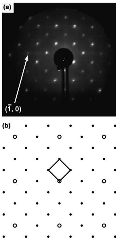
Fig. 3. (a) LEED pattern of the  $(2\sqrt{2} \times 2\sqrt{2})R45^\circ$  structure produced by annealing a  $(4 \times 13)$  oxide structure at 1000 K in vacuum. (b) Simulated LEED pattern for a  $(2\sqrt{2} \times 2\sqrt{2})R45^\circ$  unit cell. The rectangle given in (b) indicates the unit cell, and the open circles indicate the primary beams for the  $(1 \times 1)$ -Pt(100) surface.
