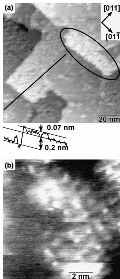
Fig. 6. STM topographs of the  $(3 \times 5)$  oxide film on Pt(100) after further oxidation using 3-L  $\text{O}_3$  with the substrate at 300 K. (a) Oxidation occurs principally at step edges (as highlighted by the superimposed black ellipse) ( $V_s = 0.47$  V,  $I_t = 0.47$  nA). The cross-section of the line scan indicated in the image is shown directly below. (b) Expanded view of a deeply oxidized domain ( $V_s = 1$  V,  $I_t = 0.48$  nA).
