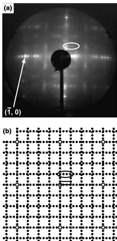
Fig. 1. (a) LEED pattern of the  $(4 \times 13)$  structure produced by 6-L  $\text{NO}_2$  oxidation of the  $(3 \times 5)$  oxide film on Pt(100) at 600 K and annealing at 950 K in vacuum. (b) Simulated LEED pattern for a  $(4 \times 13)$  unit cell. The rectangle given in (b) indicates the unit cell, and the superimposed ellipses in each figure encircle corresponding spots. The open circles indicate the primary beams for the  $(1 \times 1)$ -Pt(100) surface.
