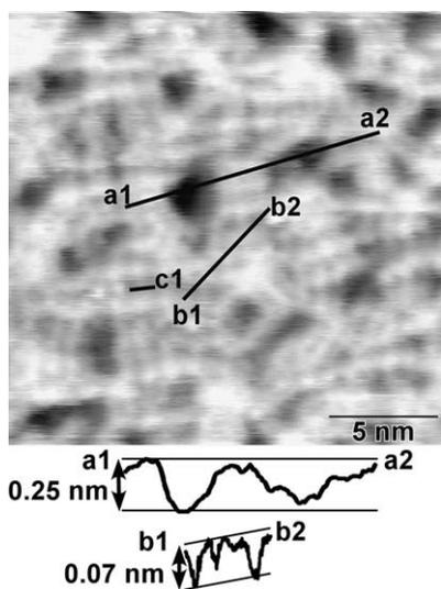
Fig. 8. STM topograph of the  $(3 \times 5)$  oxide film on Pt(100) after further oxidation using 9-L  $O_3$  with the substrate at 600 K ( $V_s = 1.1$  V,  $I_t = 0.47$  nA). Cross-sections along the lines a1–a2 and b1–b2 indicated in the image are shown directly below. A  $(2\sqrt{2} \times 2\sqrt{2})R45^\circ$ -like structure is observed (denoted as c1).
