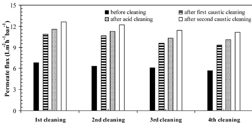
Fig. 7. Permeate flux recovery during the successive cleanings with caustic and acid solutions for the NOM-fouled membrane (as measured by DI water flux immediately after each chemical cleaning).
