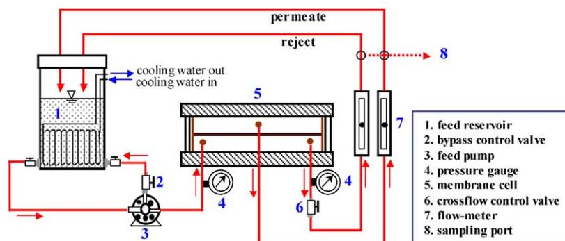
Fig. 2. Schematic diagram of the crossflow membrane filtration unit.
