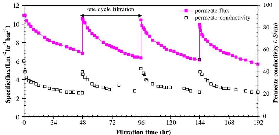
Fig. 6. Permeate flux profiles and permeate conductivity for nanofiltration tests performed with raw water using successive cleaning with caustic and acid solutions.
