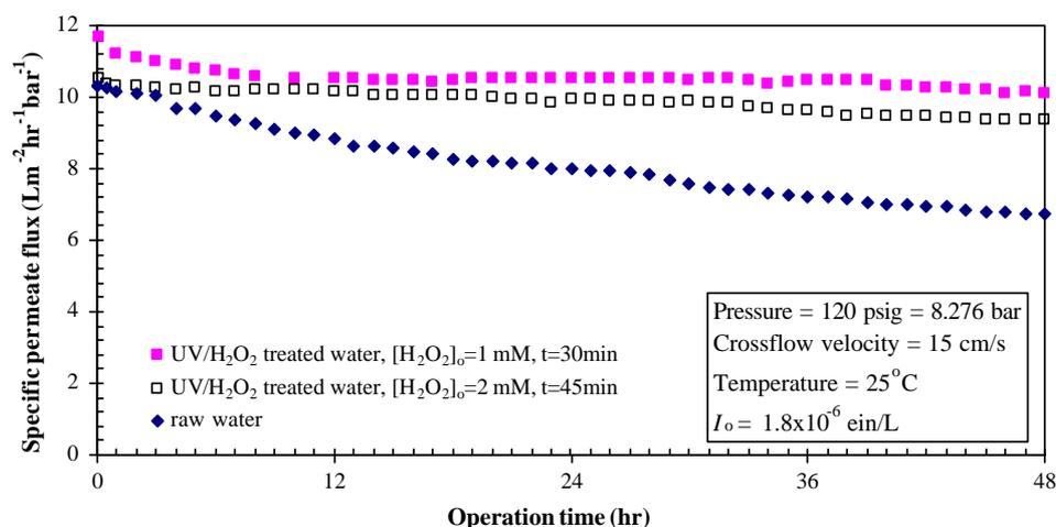
Fig. 4. Permeate flux profiles for nanofiltration performed with raw water and H<sub>2</sub>O<sub>2</sub>/UV preoxidized waters.
