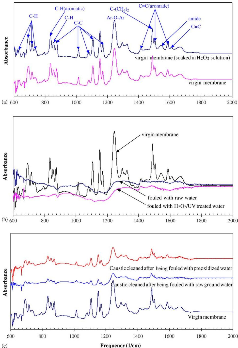
Fig. 8. The FTIR spectra of membranes at various phases of membrane operation: (a) virgin membranes, (b) fouled membranes, and (c) caustic-cleaned membranes.
