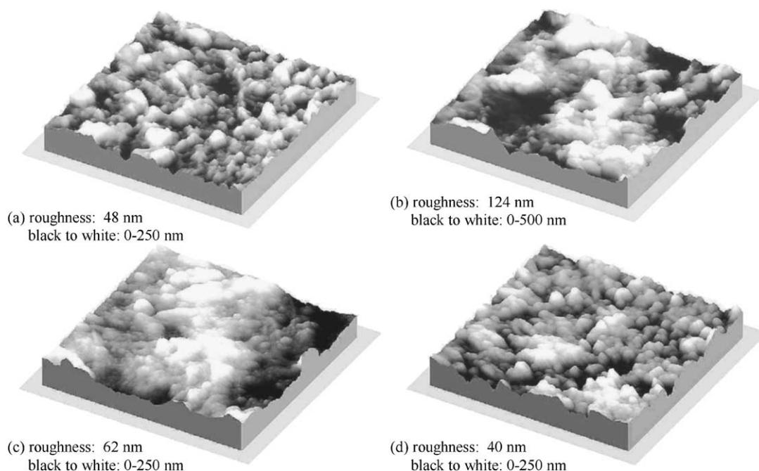
Fig. 9. AFM image scans: (a) virgin membrane (sample 1), (b) fouled with preoxidized water (sample 4), (c) surfactant-cleaned (sample 11), and (d) caustic-cleaned (sample 8).
