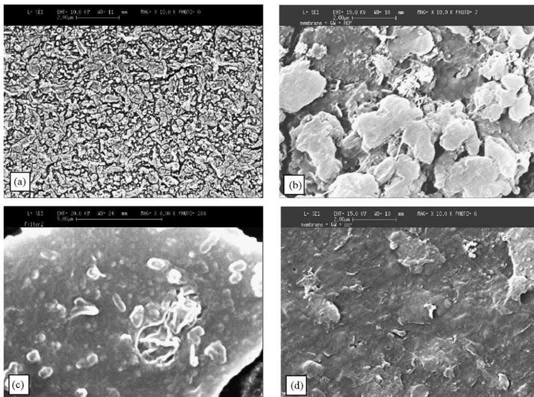
Fig. 10. Scanning electron micrographs: (a) virgin membrane (sample 1), (b) fouled with preoxidized water (sample 4), (c) fouled with raw water (sample 3), and (d) caustic-cleaned (sample 7).
