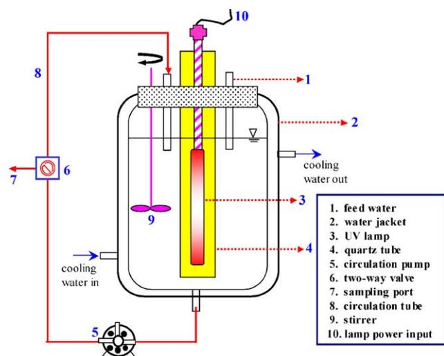
Fig. 3. Experimental setup for  $\text{H}_2\text{O}_2/\text{UV}$  pretreatment.
