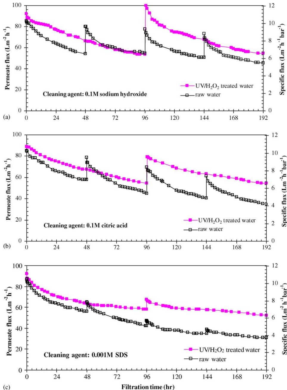
Fig. 5. Effect of the H<sub>2</sub>O<sub>2</sub>/UV pretreatment on permeate flux for various membrane cleaning strategies: (a) caustic cleaning, (b) acid cleaning, and (c) surfactant cleaning.
