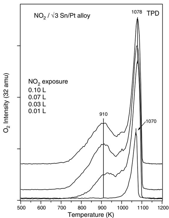
Fig. 3. O<sub>2</sub> desorption spectra resulting from NO<sub>2</sub> exposures to the  $\sqrt{3}$  Sn/Pt(1 1 1) surface alloy at 120 K.
