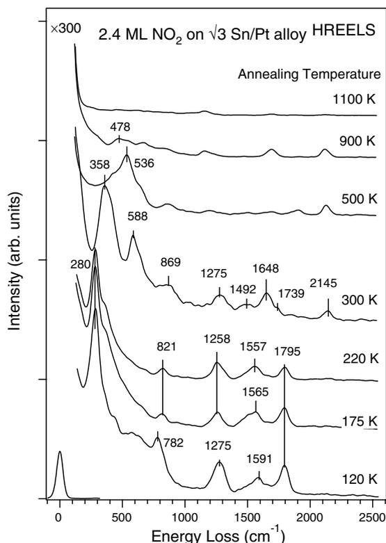
Fig. 7. HREELS warm-up experiments after 2.4 ML  $\text{NO}_2$  adsorbed on the  $\sqrt{3}$  Sn/Pt(1 1 1) alloy at 120 K. Reaction mechanism is shown on the right.
