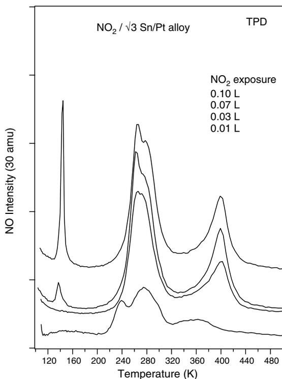
Fig. 2. NO desorption spectra resulting from NO<sub>2</sub> exposures to the  $\sqrt{3}$  Sn/Pt(1 1 1) surface alloy at 120 K.
