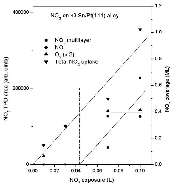
Fig. 4. Surface species concentrations as a function of  $\text{NO}_2$  exposure to the  $\sqrt{3}$  Sn/Pt(111) surface alloy at 120 K. The dashed vertical line indicates the  $\text{NO}_2$  exposure that gives a surface with a saturation monolayer coverage.
