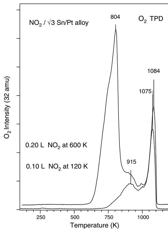
Fig. 5.  $\text{O}_2$  desorption spectra resulting from  $\text{NO}_2$  exposures on the  $\sqrt{3}$  Sn/Pt(111) surface alloy: (top) 0.20 L  $\text{NO}_2$  at 600 K; (bottom) 0.10 L  $\text{NO}_2$  at 120 K.
