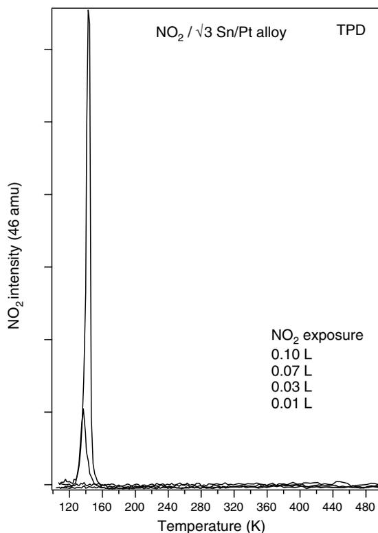
Fig. 1. NO<sub>2</sub> desorption spectra after NO<sub>2</sub> exposures on the  $\sqrt{3}$  Sn/Pt(1 1 1) surface alloy at 120 K.
