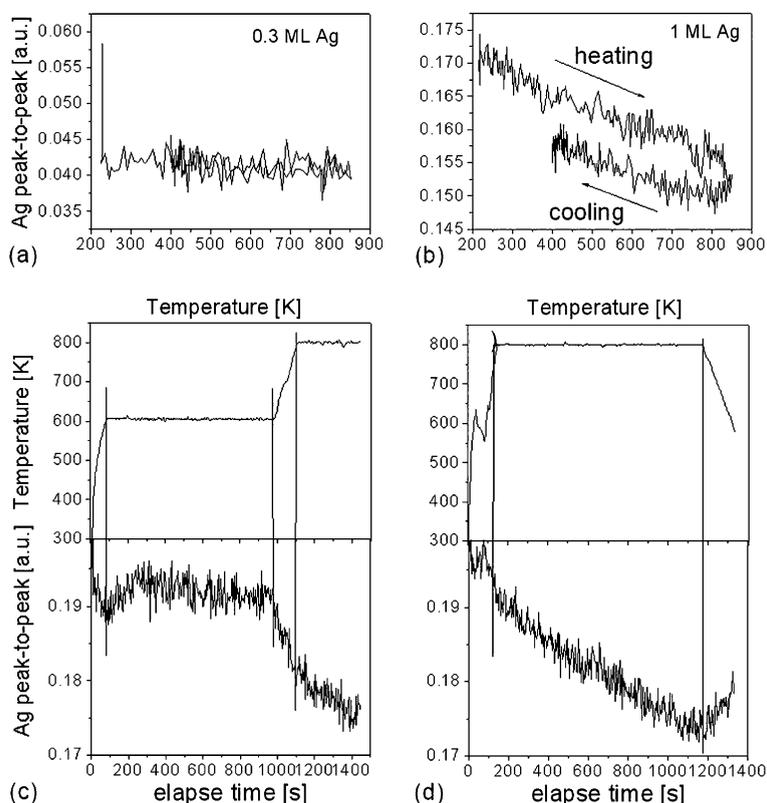
Fig. 6. Temperature-dependent AES intensities measured for (a) 0.3-ML Ag and (b) 1-ML Ag during heating at a constant rate of 1 K/s and cooling with an initial rate of 1 K/s. (c) and (d) show AES intensities measured on samples with 1-ML Ag coverage as a function of elapsed time at different temperatures. The upper graphs show the sample temperature versus time and the lower graphs show the Ag peak-to-peak AES intensities during the same time.
