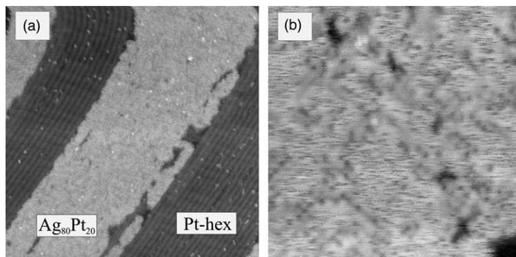
Fig. 1. STM images of submonolayer  $\text{Ag}_{80}\text{Pt}_{20}$  adislands on  $\text{Pt}(100)$  after Ag deposition at 300 K. (a) Scan area  $(60 \text{ nm})^2$ . The adislands exhibit straight edges and are separated from each other by the hex-reconstructed  $\text{Pt}(100)$  substrate. (b) Scan area  $(15 \text{ nm})^2$ . Ag is imaged brighter than Pt. This island shows a disordered structure with 20% Pt dispersed in 80% Ag.
