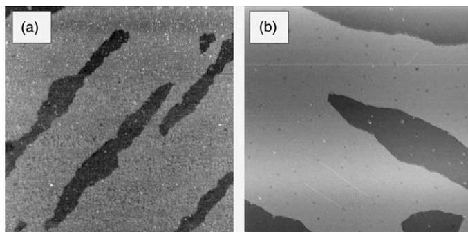
Fig. 5. STM images of (a) 0.5-ML Ag on Pt(1 0 0) annealed to 600 K. Scan area (120 nm)<sup>2</sup>. (b) 0.4-ML Ag on Pt(1 0 0) annealed to 900 K. Scan area (300 nm)<sup>2</sup>.
