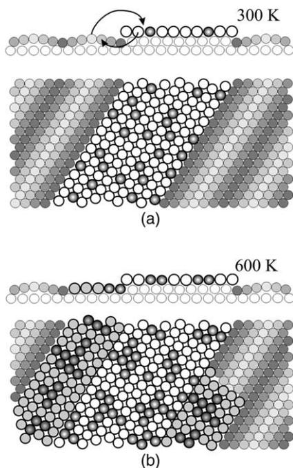
Fig. 4. Schematic illustration of spreading of the alloyed region upon annealing the sample. (a) Illustration of the island structure after growth at 300 K. (b) Ag atoms from the adislands can exchange places with Pt atoms in the lower terrace at 600 K and this results in a spreading of the alloyed region to the lower terrace.
