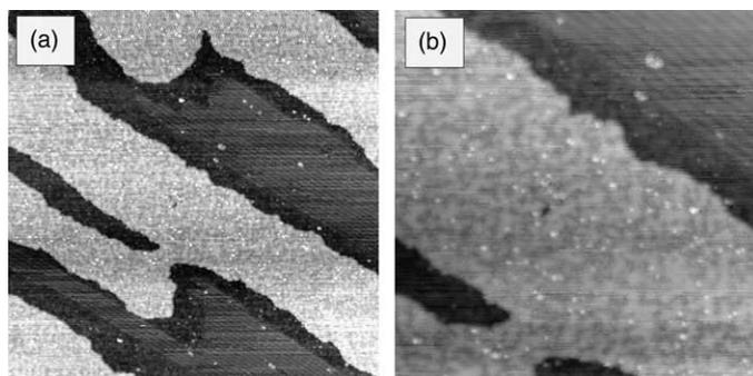
Fig. 3. STM images of a submonolayer-Ag deposit on Pt(1 0 0) after annealing to 600 K. (a) Scan area  $(110 \text{ nm})^2$  and (b) scan area  $(45 \text{ nm})^2$ . The darker (Pt) and brighter (Ag) areas in the island structure have clustered together to form a nanophasic, intermixed Ag–Pt alloy. This nanophasic morphology has spread to the lower terraces and replaced the Pt(1 0 0)-hex-reconstruction in the vicinity of the adislands.
