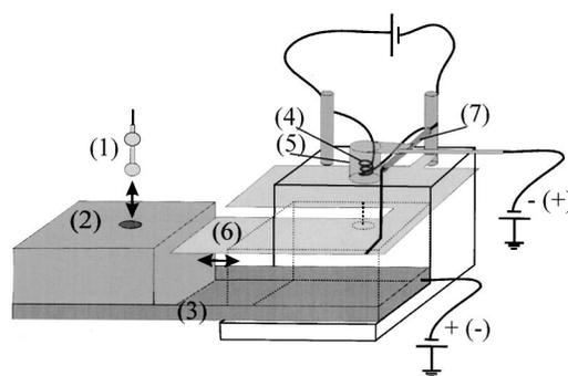
FIG. 6. STM-tip heater and sputtering device: (1) STM tip and dumbbell, (2) molybdenum block, (3) stainless-steel tray, (4) filament, (5) tantalum cylindrical shield, (6) stainless-steel foil shield, and (7) ceramic tube.
