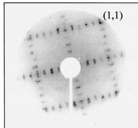
FIG. 9. LEED image at  $E_p = 56$  eV of the reconstructed Pt(100) surface showing a  $5 \times 20$  structure.
