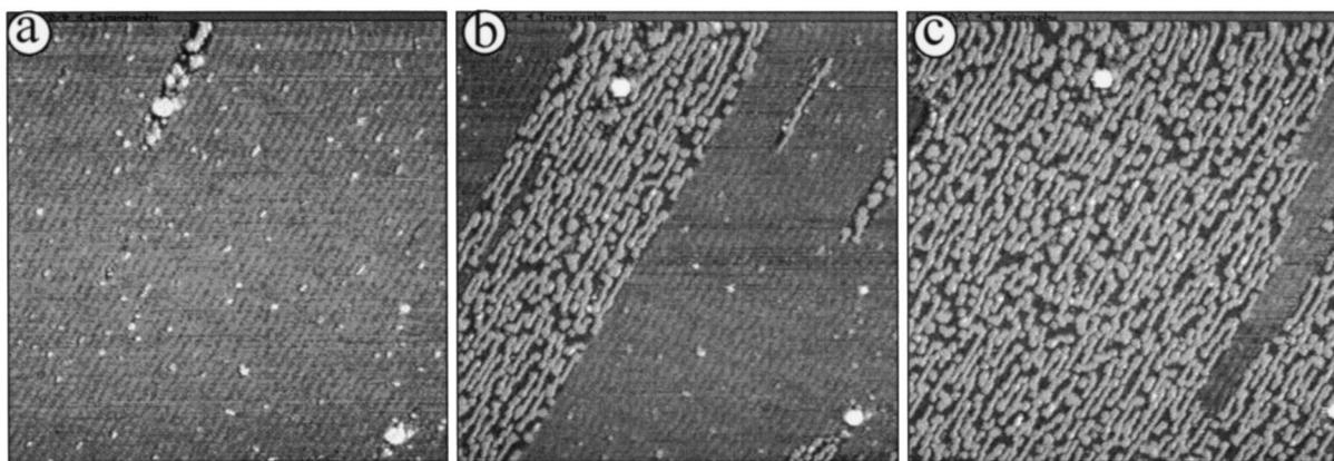
FIG. 10. Reconstructed Pt(100)-hex surface (a) prior to, (b) during, and (c) following CO adsorption. Total time was 30 min. Image size is  $60.5 \times 60.5$  nm. Tunneling conditions for all images were  $V_t = -400$  mV,  $I = 0.12$  nA.
