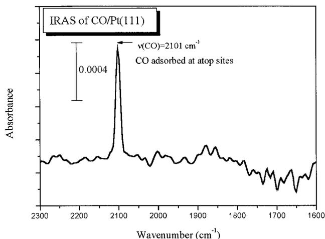
FIG. 5. FT-IRAS spectra of CO adsorbed on clean Pt(111).
