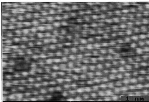
FIG. 7. Atomic resolution image of Pt(111). Image size is  $5.4 \times 4.2$  nm ( $V_t = -4.46$  V,  $I = 0.22$  nA).
