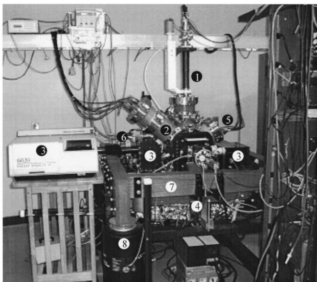
FIG. 1. Photograph of the UHV-STM chamber. (1) STM transfer-rod bellows, (2) CMA, (3) FT-IRAS mirror and detector purge boxes, (4) QMS, (5) LEED optics, (6) cryostat cold finger, (7) wooden beam frame, and (8) laminar flow air legs.
