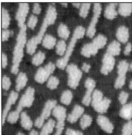
FIG. 11. Unreconstructed Pt(100) surface with adsorbed  $c(2 \times 2)$ -CO layer. Image size is  $16.6 \times 16$  nm ( $V_t = -95$  mV,  $I = 0.18$  nA).
