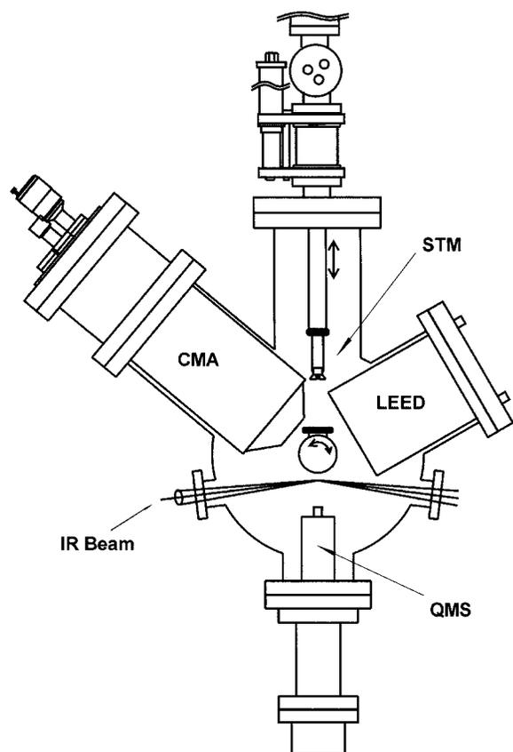
FIG. 2. Cross section of the chamber in the surface analysis plane showing the instrumentation.
