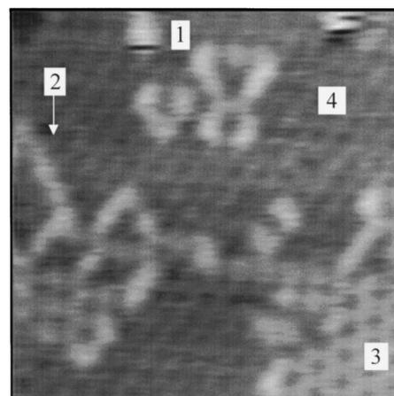
FIG. 8. Sn/Pt(111) surface alloy showing (1) defect sites, (2) antiphase boundary, (3) ordered  $(2 \times 2)$  region, and (4) ordered  $(\sqrt{3} \times \sqrt{3})R30^\circ$  domain. Image size is  $7.5 \times 7.6$  nm ( $V_t = -276$  mV,  $I = 0.46$  nA).
