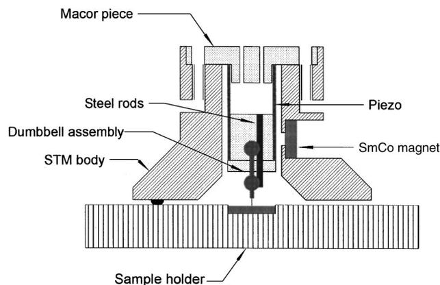
FIG. 4. Cross section of STM head. The dumbbell and tip assembly is held against the rods by a SmCo magnet. Course approach is accomplished by application of a cycloid voltage waveform to the  $z$  component of the piezo.
