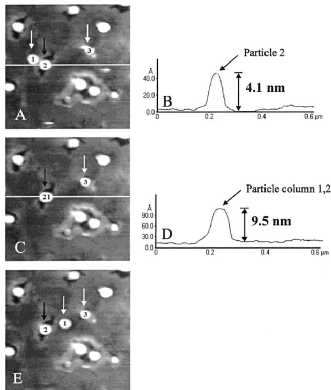
**Figure 4.** SFM images and corresponding line scans displaying the successful construction of a two-particle, upright column by pushing particle "1" on top of particle "2". The scan size is 600 × 600 nm<sup>2</sup>, and the height scale is 6 nm from black to white.
