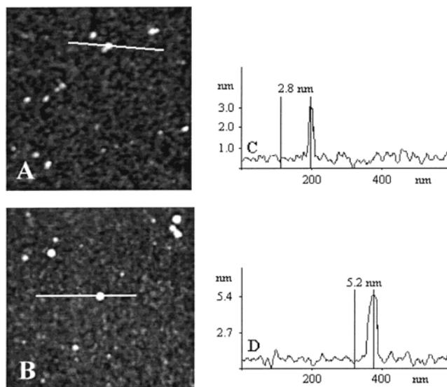
**Figure 1.** Sequence of  $500 \times 500 \text{ nm}^2$  SFM images displaying areas of a SiO<sub>2</sub>/nanoparticle sample: A, after deposition of an ODS layer; B, after oxidation of the hydrocarbon present in ODS. The change in the height of the particles is displayed in the corresponding linescans C and D. The scan size is  $1 \times 1 \mu\text{m}^2$  and the height scale in the images is (A) 2 nm and (B) 3.5 nm from black to white, respectively.
