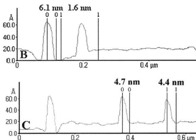
**Figure 3.** SFM image, A, and corresponding line scans, B and C, recording the embedding of Au nanoparticles in layers of SiO<sub>2</sub> by successive ODS deposition and oxidation cycles. The maximum height difference between uncovered and covered areas was measured to be 1.6 nm, corresponding to six layers of SiO<sub>2</sub>. The scan size is  $500 \times 500$  nm<sup>2</sup>, and the height scale is 3 nm from black to white.
