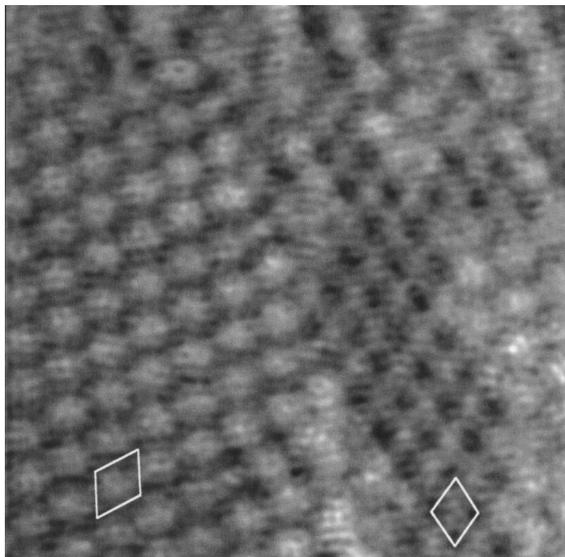
Fig. 1. STM image of  $p(2 \times 2)$  (left) and  $(\sqrt{3} \times \sqrt{3})R30^\circ$  (right) domains of an Sn–Pt (111) surface alloy. The imaged unit cells of the ordered alloys are also indicated (see also Fig. 3). Scan area:  $6.3 \times 6.3 \text{ nm}^2$ ; tunneling conditions are  $U_{\text{Bias}} = 2.5 \text{ mV}$ ,  $I = 2 \text{ nA}$ .
