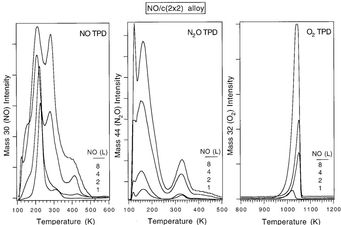
Figure 5. NO, N<sub>2</sub>O, and O<sub>2</sub> TPD traces obtained after NO exposures on the c(2 × 2) Sn/Pt(100) alloy at 100 K.
