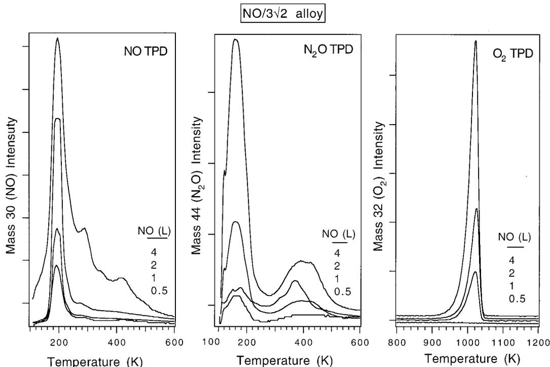
**Figure 7.** NO, N<sub>2</sub>O, and O<sub>2</sub> TPD traces obtained following NO exposures on the (3√2 × √2)R45°Sn/Pt(100) alloy at 100 K.
