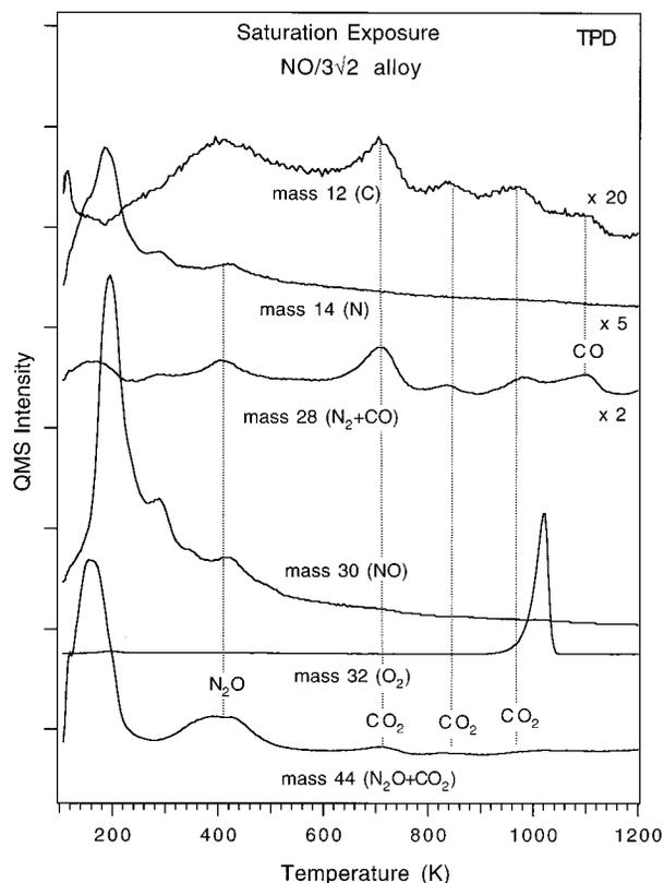
Figure 6. TPD curves from an NO monolayer on the (3√2 × √2)-R45°Sn/Pt(100) alloy at 100 K.
