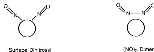
**Figure 15.** Schematic representation of models for (a) monomeric NO species adsorbed at different sites and (b) dimeric NO species adsorbed as surface dinitrosyl and  $(NO)_2$  dimer configuration.
