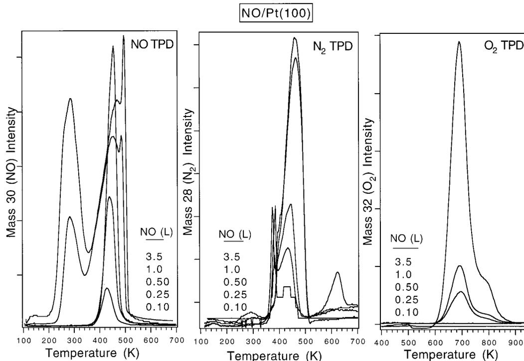
**Figure 2.** NO, N<sub>2</sub>, and O<sub>2</sub> TPD traces following NO exposures on the hex-Pt(100) surface.
