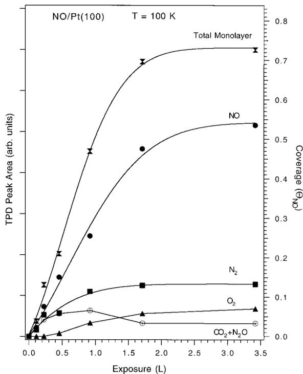
**Figure 3.** Uptake curves constructed from TPD results detailing NO adsorption kinetics on hex-Pt(100) at 100 K. The value for  $\theta_{\text{NO}}^{\text{sat}}$  on Pt(100) was set to 0.73 ML.<sup>29</sup>
