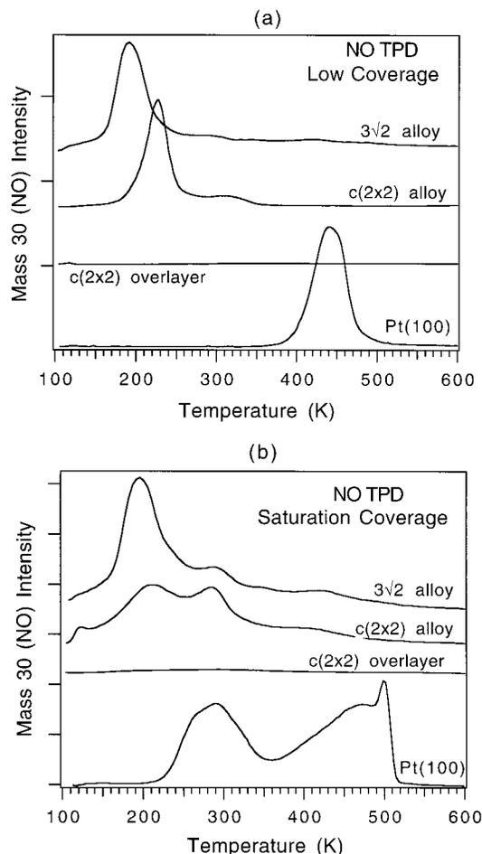
**Figure 9.** Comparison of NO TPD results from hex-Pt(100), the two alloys, and a  $c(2 \times 2)$  overlayer at two coverages of NO (a)  $\theta_{\text{NO}} = 0.1$  and (b)  $\theta_{\text{NO}} = \theta_{\text{NO}}^{\text{sat}}$  at 100 K on each surface.
