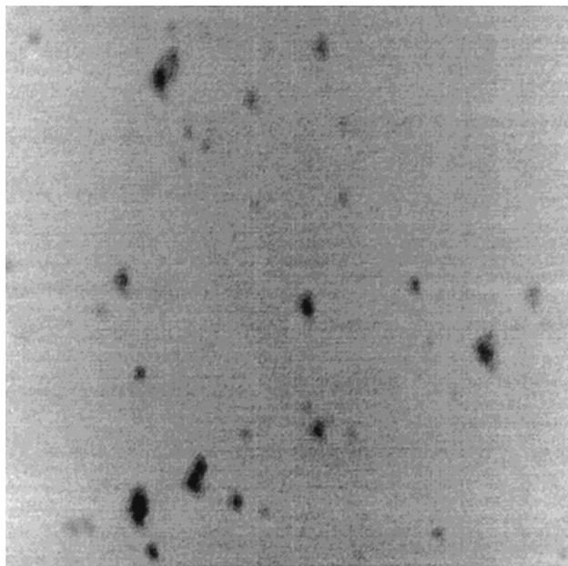
**Figure 2.** Dynamic SFM image of a barite (001) surface after dissolution in 0.5 M HCl for 10 s. Image size is  $1 \mu\text{m} \times 1 \mu\text{m}$ . Depth scale from black to white is 2.5 nm.
