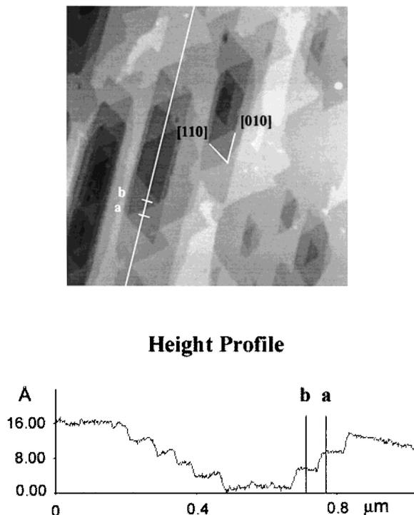
**Figure 7.** (top) Dynamic SFM image of a barite (001) surface following dissolution in 0.18 M EDTA for 5 min. (bottom) A line profile taken across a pit along the *b* axis. The morphology of etch pits was defined by monolayer steps parallel to the [010] and [110] directions. Flat terraces at the bottoms of the etch pits were observed. The height difference between the two terraces denoted as *a* and *b* is 3.61 Å. Image size is 1 μm × 1 μm. Depth scale from black to white is 4 nm.
