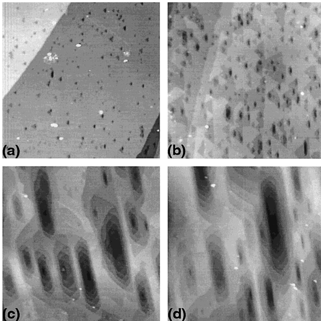
**Figure 6.** Dynamic SFM images of a barite (001) surface after dissolution in 0.18 M EDTA for (a) 1, (b) 3, (c) 10, and (d) 40 min. Image size is  $1.5 \mu\text{m} \times 1.5 \mu\text{m}$ . Depth scale from black to white is (a) 3, (b) 4, (c) 8, and (d) 12 nm.
