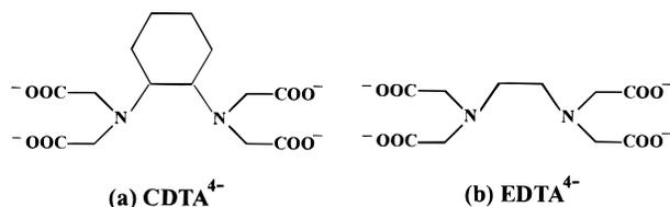
**Figure 1.** Molecular structures of polyaminoacetate scale dissolvers: (a) CDTA<sup>4-</sup>; (b) EDTA<sup>4-</sup>.
