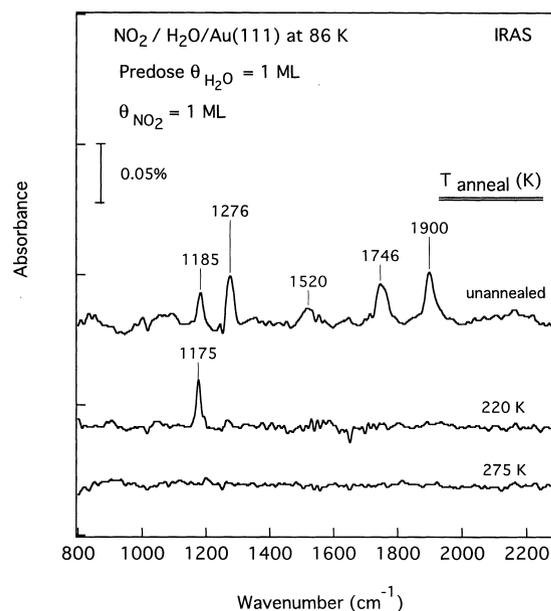
Fig. 7. IRAS 'warm-up' spectra obtained after sequentially heating the substrate to the indicated annealing temperatures. A 1 ML NO<sub>2</sub> exposure was given on an ice monolayer film on Au(111) at 86 K, and then the substrate was annealed to the indicated temperature for 30 s. All of the spectra were collected with the substrate at 86 K.
