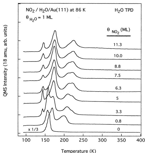
Fig. 1.  $\text{H}_2\text{O}$  TPD spectra following  $\text{NO}_2$  exposures on an ice monolayer film on a Au(111) surface at 86 K. The bottom trace is for  $\text{H}_2\text{O}$  desorption from a 1 ML  $\text{H}_2\text{O}$  film on Au(111), in the absence of  $\text{NO}_2$  coadsorption.
