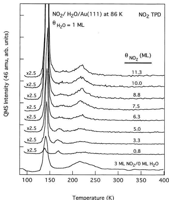
Fig. 2.  $\text{NO}_2$  TPD spectra following  $\text{NO}_2$  exposures on an ice monolayer film on a Au(111) surface at 86 K. The bottom TPD spectrum is for  $\text{NO}_2$  desorption from a 3 ML  $\text{NO}_2$  exposure on the Au(111) surface, in the absence of  $\text{H}_2\text{O}$  coadsorption.
