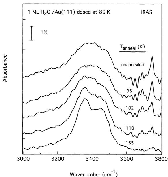
Fig. 6. IRAS spectra obtained after dosing 1 ML H<sub>2</sub>O on a Au(111) surface at 86 K and then annealing the ice monolayer film to the indicated temperature for 30 s. All of the spectra were collected with the substrate at 86 K.
