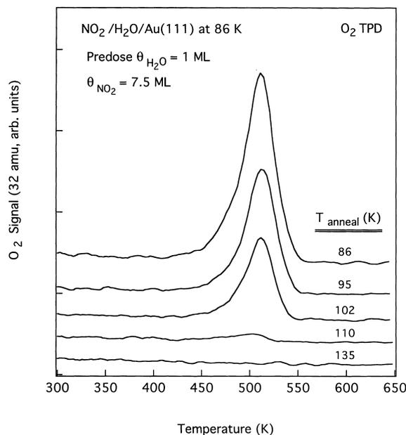
Fig. 5.  $O_2$  TPD spectra following 7.5 ML  $NO_2$  exposures on ice monolayer films on Au(111) at 86 K. The important variable probed is the preannealing temperature of the ice films prior to  $NO_2$  exposures. Following the deposition of 1 ML  $H_2O$  on a Au(111) surface at 86 K, the substrate was annealed to the indicated temperature for 30 s, and then exposed to  $NO_2$  with the substrate at 86 K.
