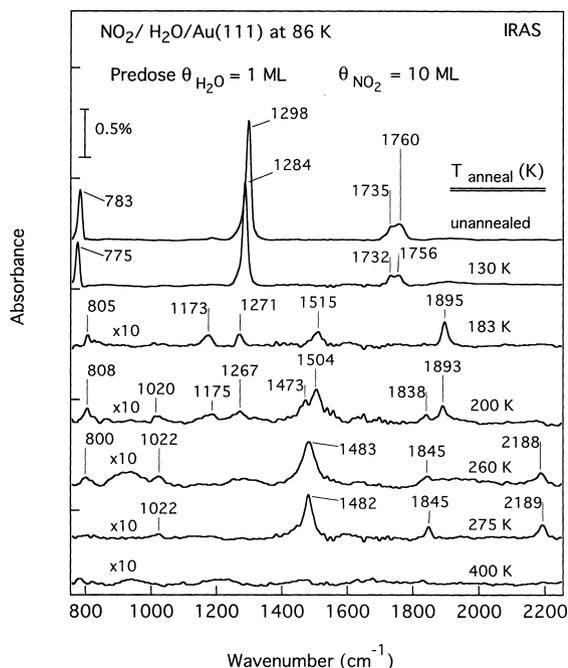
Fig. 8. IRAS ‘warm-up’ spectra obtained after sequentially heating the substrate to the indicated annealing temperatures. A 10 ML  $NO_2$  exposure was given on an ice monolayer film on Au(111) at 86 K, and then the substrate was annealed to the indicated temperature for 30 s. All of the spectra were collected with the substrate at 86 K.
