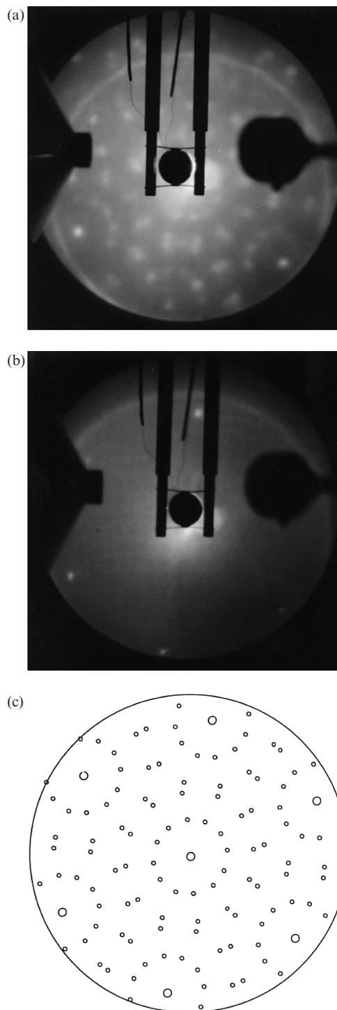
Fig. 3. LEED observations for  $C_{60}$  films deposited on Pt(111) at 300 K, after heating to (a) 900 K, (b) 1000 K; (c) schematic explanation of the LEED [18]. All images are at  $E_p = 65$  eV.
