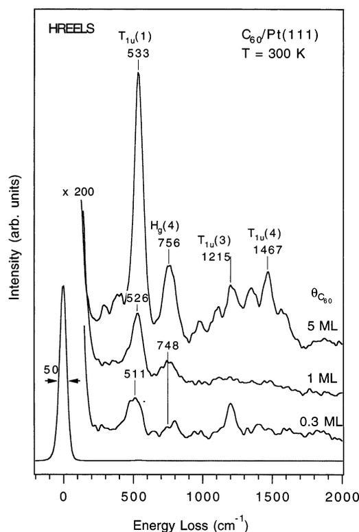
Fig. 1. HREELS spectra of  $C_{60}$  deposited on Pt(111) at 300 K.
