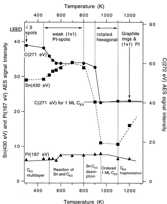
Fig. 5. AES studies of multilayer  $C_{60}$  films (4 ML) following annealing on the  $(\sqrt{3} \times \sqrt{3})R30^\circ$  surface alloy in the 300–1200 K temperature range. LEED observations are given in the top panel, followed by corresponding AES intensities of the C(271 eV), Sn(430 eV) and Pt(167 eV) signals.
