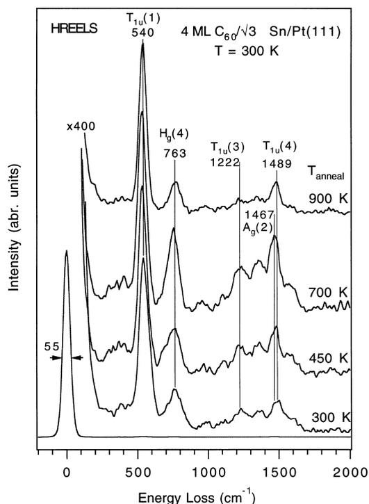
Fig. 6. HREELS spectra for 4 ML  $C_{60}$  deposited on  $(\sqrt{3} \times \sqrt{3})R30^\circ$  Sn/Pt(111) surface alloy at 300 K, following sequential annealing to temperatures up to 900 K.
