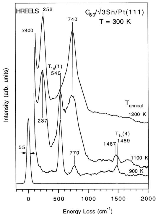
Fig. 8. HREELS spectra after high temperature annealing of the ordered  $C_{60}$  monolayer, produced by heating multilayer  $C_{60}$  films on the  $\sqrt{3}$  Sn/Pt(111) surface alloy to 900 K. Extensive fragmentation of  $C_{60}$  occurs at  $T \geq 1100$  K, and is nearly complete by 1200 K.
