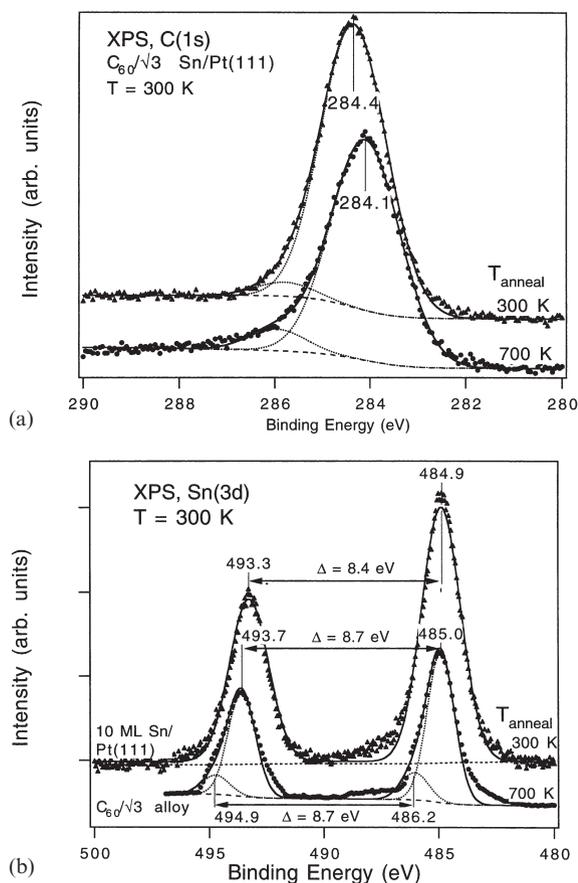
Fig. 7. XPS spectra of (a) C(1s) (b) Sn(3d) core levels, for 4 ML  $C_{60}$  deposited on  $(\sqrt{3} \times \sqrt{3})R30^\circ$  Sn/Pt(111) surface alloy at 300 K, after annealing this film to 700 K. The C(1s) level shows a 0.3 eV chemical shift to lower BE. In comparison with thick Sn films, the Sn(3d) levels show some broadening, which causes small increases in BE and in the splitting of the levels.
