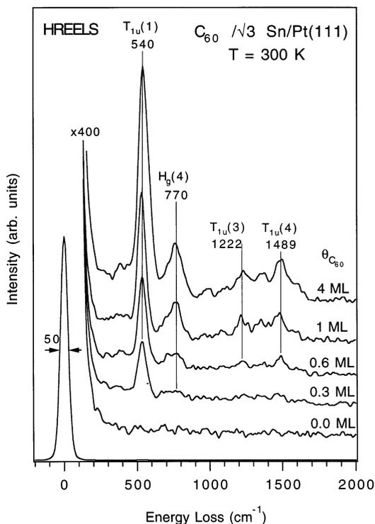
Fig. 2. HREELS spectra of  $C_{60}$  deposited on  $(\sqrt{3} \times \sqrt{3})R30^\circ$  Sn/Pt(111) surface alloy at 300 K.
