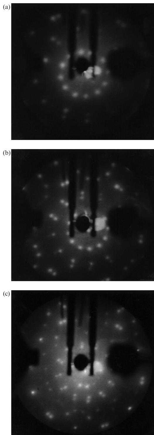
Fig. 4. LEED observations for  $C_{60}$  films deposited on the  $(\sqrt{3} \times \sqrt{3})R30^\circ$  Sn/Pt(111) surface alloy at 300 K, after heating to 900 K. The LEED spectra were obtained at an  $E_p$  of (a) 25 eV, (b) 35 eV and (c) 65 eV. No change in the pattern occurs after heating up to 1100 K.
