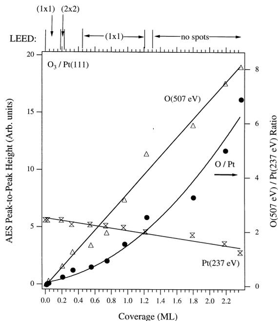
Fig. 5. AES intensities and the O(507)/Pt(237) AES ratio are shown as a function of oxygen coverage,  $\theta_O$ , as determined by  $O_2$  TPD peak areas. The result of concurrent LEED measurements are shown along the top bar.
