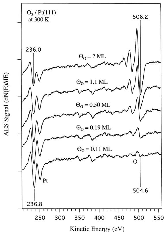
Fig. 6. AES spectra for increasing  $O_3$  exposures on Pt(111) at 300 K. Shifts of the Pt and O AES peaks indicate changes in chemical state due to oxidation.
