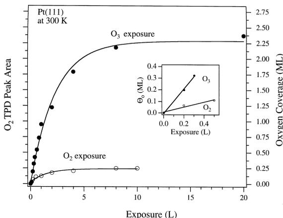
Fig. 4. Oxygen uptake curves comparing the efficiency of  $O_3$  and  $O_2$  exposures on Pt(111) at 300 K. The inset shows details for oxygen accumulation from  $O_3$  and  $O_2$  at low exposures.
