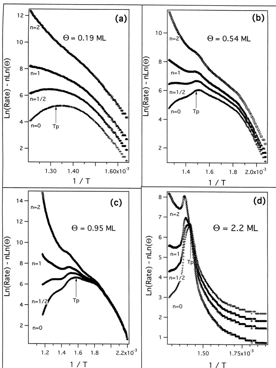
Fig. 3. Arrhenius plots of the  $\text{O}_2$  TPD curves for oxygen concentrations of (a) 0.19, (b) 0.54, (c) 0.95 and (d) 2.2 ML using the method of Parker et al. [31]. For the several curves shown here, a straight line was obtained when  $n=2$  for  $\theta_o=0.19$  ML, but for the other coverages shown, no choice of  $n=0-2$  gave linear plots over the entire desorption range.
