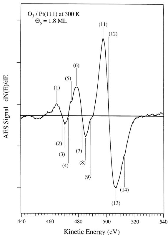
Fig. 7. O (KVV) lineshape for  $\theta_{\text{O}}=1.8$  ML on Pt(111). The features denoted by labels correspond to characteristics in the lineshape used to derive chemical state information, specifically the presence of oxidic oxygen.
