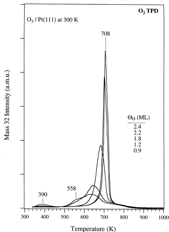
Fig. 2.  $\text{O}_2$  TPD curves following  $\text{O}_3$  exposures of 1 to 20 L on Pt(111) at 300 K.
