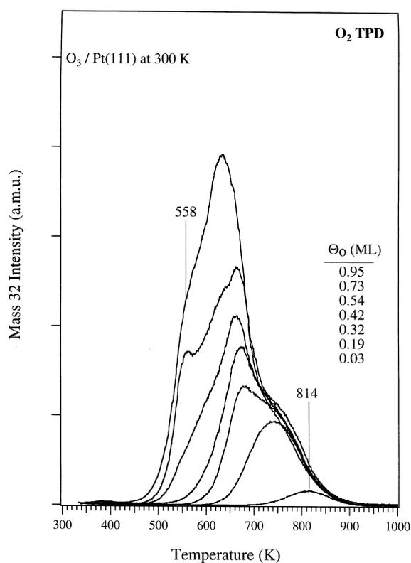
Fig. 1.  $\text{O}_2$  TPD curves after  $\text{O}_3$  exposures of 0.1–1 L on Pt(111) at 300 K. The coverages denoted as  $\theta_{\text{O}}$  were calibrated by using the  $\text{O}_2$  TPD area following saturation exposures of  $\text{O}_2$  to be  $\theta_{\text{O}}=0.25$  ML [3].
