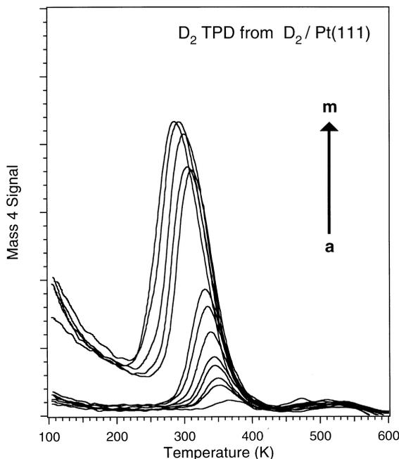
Fig. 1.  $D_2$  TPD spectra after  $D_2$  adsorption on Pt(111) at 110 K.  $D_2$  exposures are from the cold (room temperature) Pt tube doser to give a background pressure of  $10^{-8}$  Torr: (a) 0 L, (b) 0.05 L, (c) 0.10 L, (d) 0.15 L, (e) 0.20 L, (f) 0.40 L, (g) 0.70 L, (h) 1.00 L. Exposures at  $10^{-7}$  Torr: (i) 2.5 L, (j) 5 L, (k) 12.5 L, (l) 125 L, (m) 250 L.
