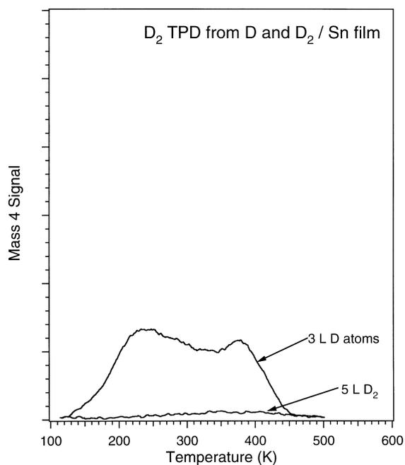
Fig. 5.  $D_2$  TPD spectra after exposures of  $D_2$  (bottom curve) and D atoms (top curve) on a thin S film at 110 K.
