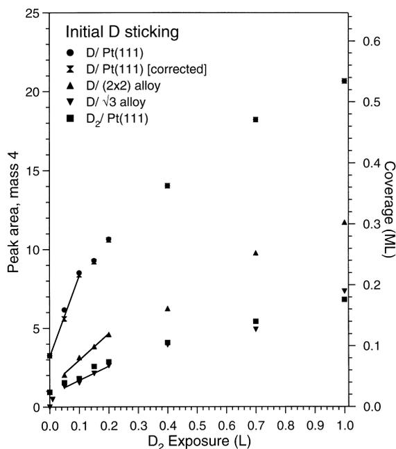
Fig. 6. Adsorbed D uptake curve from integrating the D<sub>2</sub> TPD in the low coverage range. Values for the initial sticking coefficients  $S_0$  of D atoms on each surface were obtained by fitting a straight line to the low coverage data for  $\theta_D > 0.05$  ML.
