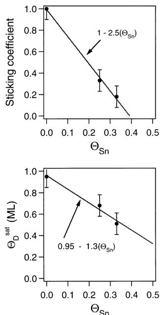
Fig. 8. Influence of alloyed Sn surface atoms on the uptake kinetics for incident D atoms compared to values on Pt(111). Top: initial sticking coefficient,  $S_0$ . Bottom: saturation coverage of adsorbed D,  $\theta_D^{sat}$ .
