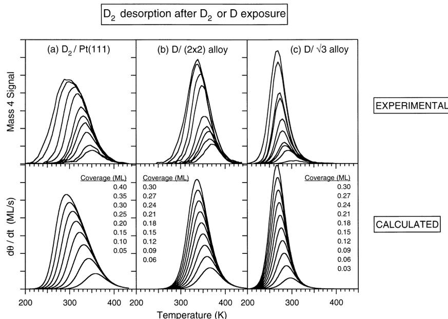
Fig. 10. Experimental (top) and simulated (bottom) TPD spectra for D<sub>2</sub> desorption. Simulation were performed using Eq. (1) with  $n=2$ .
