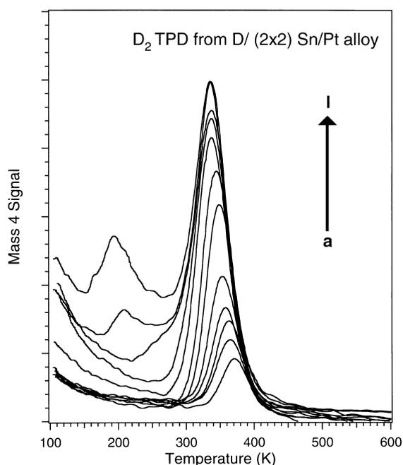
Fig. 3.  $D_2$  TPD spectra after D adsorption on the  $p(2 \times 2)$  Sn/Pt(111) surface at 110 K. Exposures at  $10^{-8}$  Torr: (a) 0 L, (b) 0.01 L, (c) 0.05 L, (d) 0.10 L, (e) 0.15 L, (f) 0.20 L, (g) 0.40 L, (h) 0.70 L, (i) 1.00 L. Exposures at  $10^{-7}$  Torr: (j) 1.3 L, (k) 2.6 L, (l) 6.5 L. Exposures at  $10^{-6}$  Torr: (m) 26 L, (n) 130 L.
