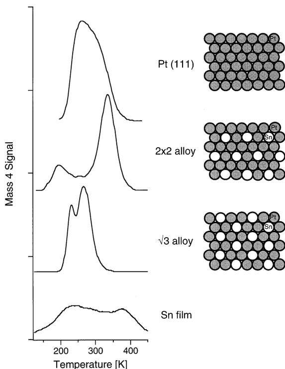
Fig. 9. Comparison of the  $D_2$  TPD spectra obtained for saturation coverages of adsorbed D produced by incident D atoms on several surfaces at 110 K.
