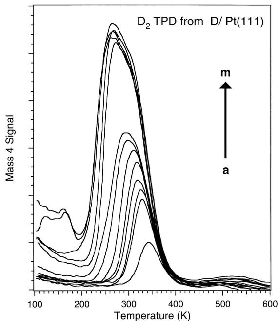
Fig. 2.  $D_2$  TPD spectra after D atom exposures on Pt(111) at 110 K. Relative D atom exposures ( $T_{\text{Pt tube}} = 1300 \text{ K}$ ) as measured by the  $D_2$  background gas at  $10^{-8}$  Torr: (a) 0 L, (b) 0.05 L, (c) 0.10 L, (d) 0.15 L, (e) 0.20 L, (f) 0.40 L, (g) 0.70 L, (h) 1.00 L. Exposures at  $10^{-7}$  Torr: (i) 2.5 L, (j) 5 L, (k) 12.5 L, (l) 25 L, (m) 50 L.
