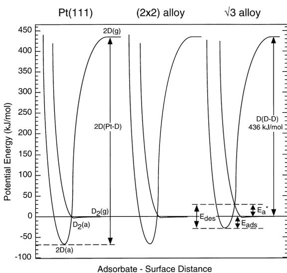
Fig. 11. Two-dimensional potential energy curves for dissociative D<sub>2</sub> chemisorption on Pt(111) and the two ordered surface alloys.
