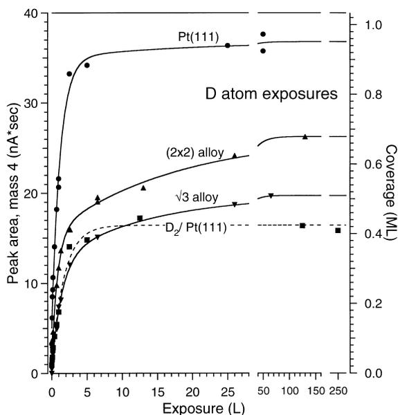
Fig. 7. Adsorbed D uptake curves over the full coverage range, showing the saturation coverages of adsorbed D on the three surfaces. As a reference, the adsorbed D uptake curve (dashed line) from  $D_2$  exposures on Pt(111) at 110 K is also shown.
