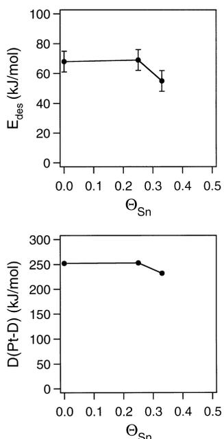
Fig. 12. Influence of alloyed Sn surface atoms on the  $\text{D}_2$  desorption energetics (top curve) and Pt–D bond strength (bottom curve) compared to values on Pt(111).
