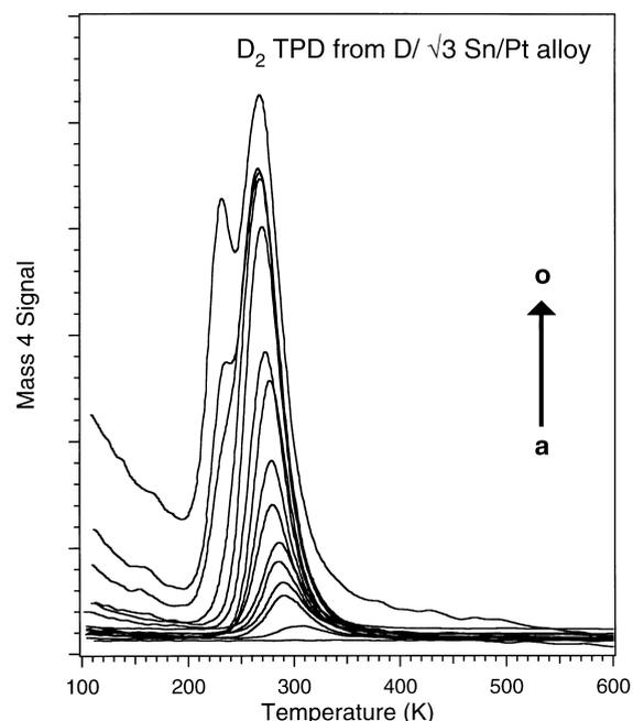
Fig. 4.  $D_2$  TPD spectra after D adsorption on the  $(\sqrt{3} \times \sqrt{3})R30^\circ$  Sn/Pt(111) surface at 110 K. Exposures at  $10^{-8}$  Torr: (a) 0 L, (b) 0.01 L, (c) 0.05 L, (d) 0.10 L, (e) 0.15 L, (f) 0.20 L, (g) 0.40 L, (h) 0.70 L, (i) 1.00 L. Exposures at  $10^{-7}$  Torr: (j) 1.3 L, (k) 2.6 L, (l) 6.5 L, (m) 13 L, (n) 26 L. Exposures at  $10^{-6}$  Torr: (o) 65 L.
