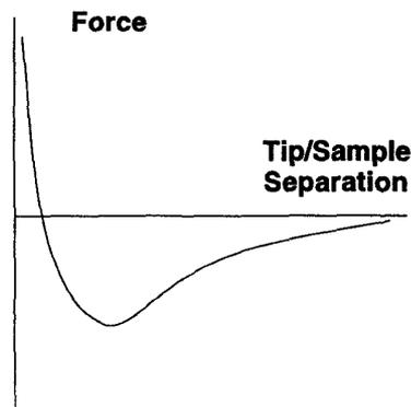
Figure 2 – Typical force between tip and sample as a function of their distance.
