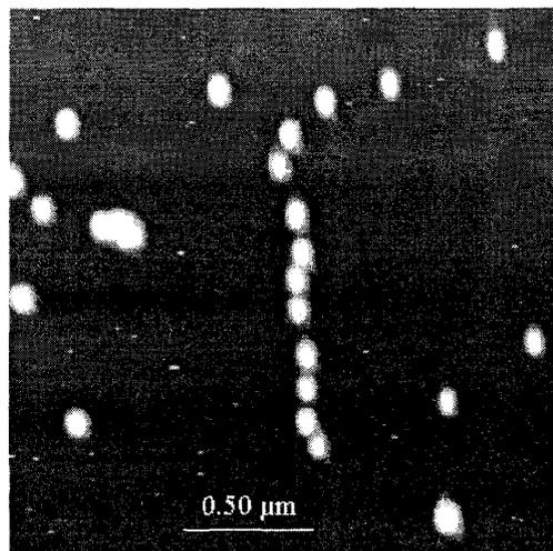
Figure 3 – A line pattern of Au balls on mica.
