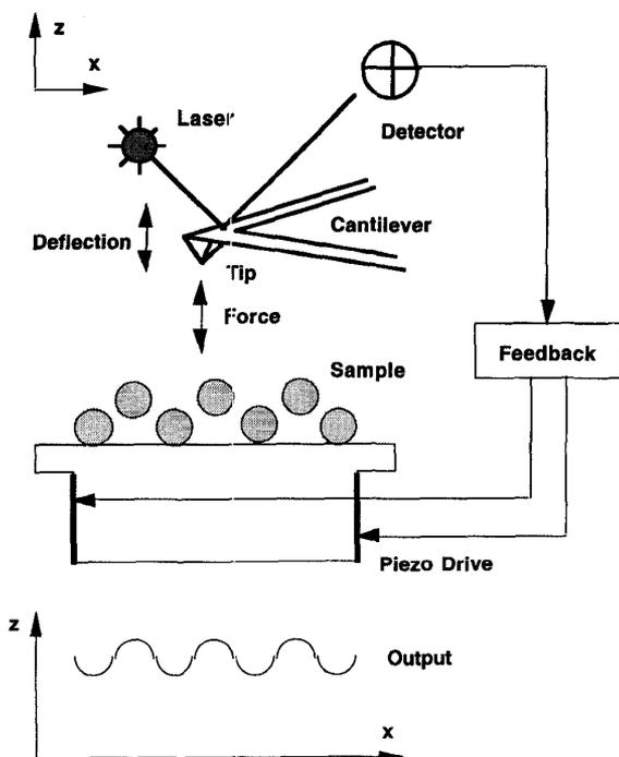
Figure 1 – Principles of operation of the AFM (not to scale).
