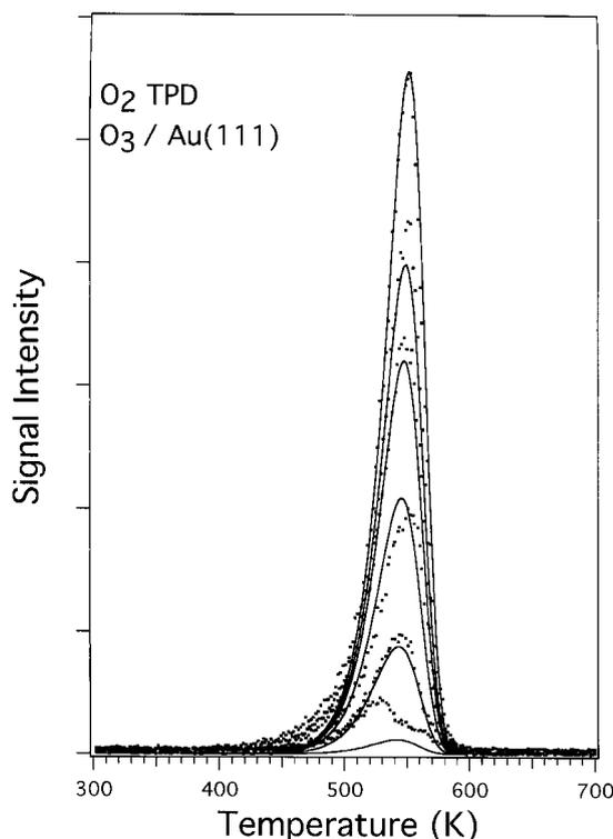
Fig. 7. Computer simulation (solid curve) of the TPD data (points) in Fig. 5. This simulation used a Polanyi–Wigner form of the desorption rate equation with first-order kinetics, a value of  $5.5 \times 10^{11} \text{ s}^{-1}$  for the pre-exponential factor, and a coverage-dependent activation energy of  $E_d = 30 + 0.75(H_0/H_{0\text{max}})$  ( $\text{kcal mol}^{-1}$ ), with  $H_{0\text{max}} = 1.2 \text{ ML}$ .
