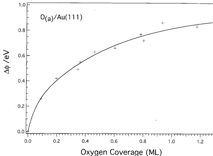
Fig. 3. Work function change  $\Delta\phi$  measured as a function of oxygen coverage. The solid curve is a fit for the data using Eq. (1).
