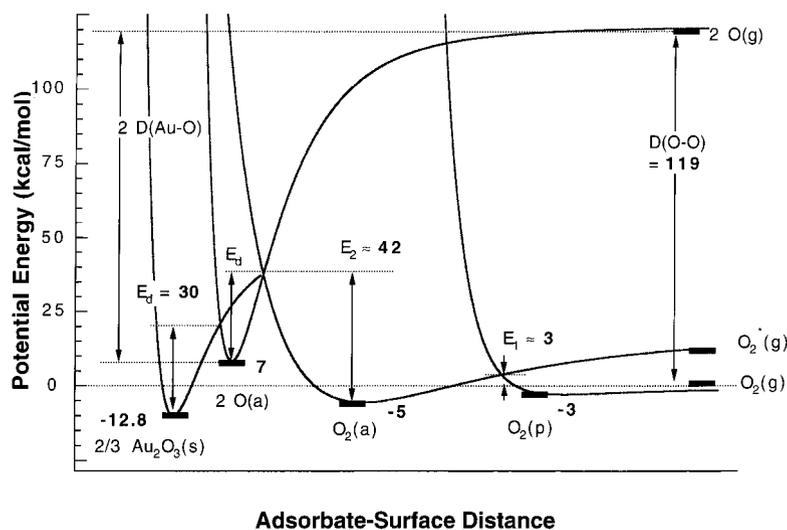
Fig. 8. Schematic potential energy diagram of the oxygen interaction with Au(111). Values for the heats of formation of gaseous, adsorbed and oxidic species are indicated by solid bars.
