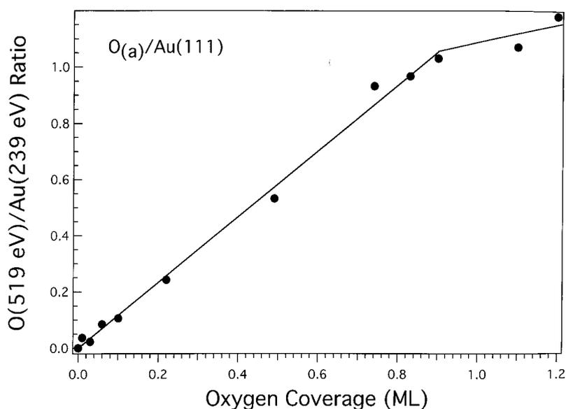
Fig. 1. Peak-to-peak height ratio for O(519 eV)/Au(239 eV) in AES for increasing oxygen coverage as determined from  $O_2$  TPD integrated areas, on Au(111) at 300 K.
