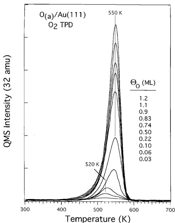
Fig. 5. Oxygen TPD following increasing exposures of ozone on Au(111) at 300 K. The oxygen coverages indicated were determined from the ratio of the integrated area under the peaks to that of the largest curve for which  $H_0 = 1.2$  ML.
