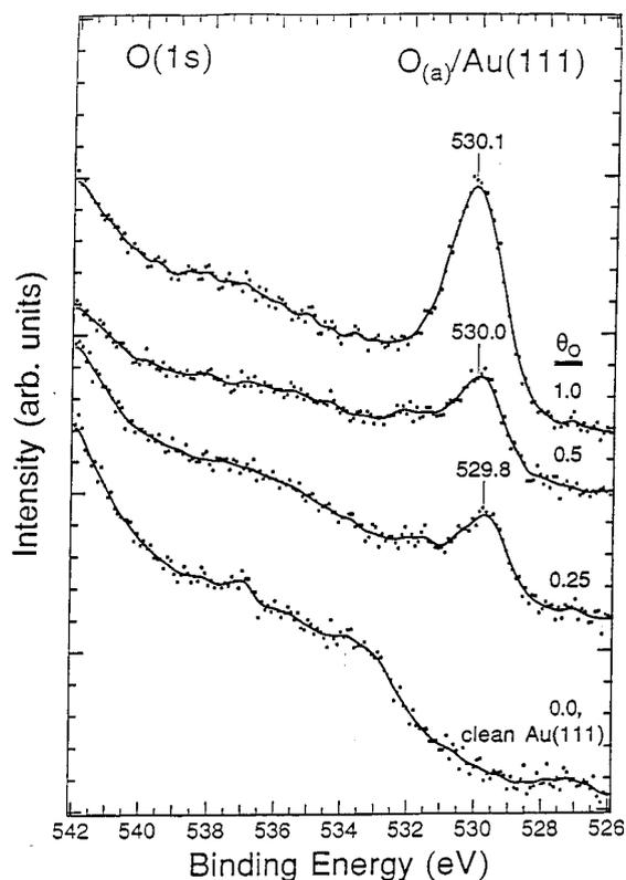
Fig. 4. O 1s XPS spectra after ozone exposure on clean Au(111) at 300 K. The oxygen coverages were determined by AES. (Taken from Ref. [29].)
