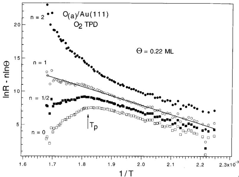
Fig. 6. Oxygen TPD curves for  $H_0 = 0.22 \text{ ML}$  plotted using the method of Parker et al. [58]. Plots for several choices of  $n$ , the desorption kinetic order, are shown, and only the data for  $n=1$  can be described well by a line in the region of  $T_p$ .
