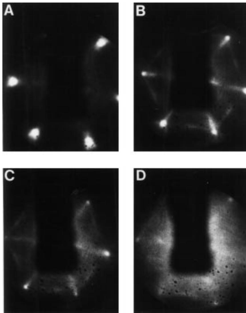
Fig. 2. LEED photographs taken at several oxygen coverages using an incident beam energy of  $\sim 66$  eV. (A) Clean Au(111), (B) 0.22 ML, (C) 0.5 ML and (D) 1.2 ML.
