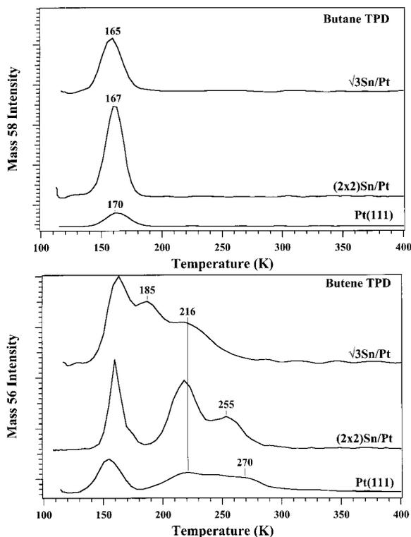
Fig. 10. Butane and butene TPD spectra after a methylacetylene submonolayer and saturation exposure on the Pt(111),  $(2 \times 2)$  and  $\sqrt{3}$  Sn/Pt(111) surface alloys at 108 K.
