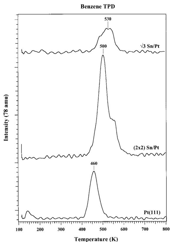
Fig. 11. Benzene TPD spectra after a methylacetylene saturation exposure on the Pt(111),  $(2 \times 2)$  and  $\sqrt{3}$  Sn/Pt(111) surface alloys at 108 K.
