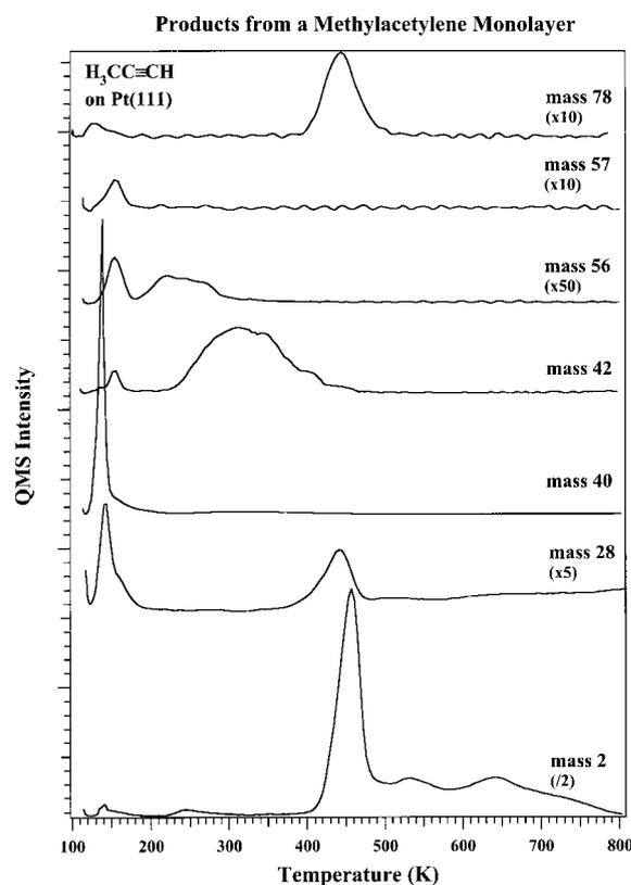
Fig. 6. TPD spectra of products from the reaction of methylacetylene after the adsorption of a coverage slightly greater than 1 ML of methylacetylene dosed at 108 K on the Pt(111) surface.
