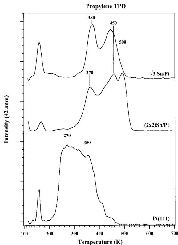
Fig. 9. Propylene TPD spectra after a methylacetylene saturation exposure on the Pt(111),  $(2 \times 2)$  and  $\sqrt{3}$  Sn/Pt(111) surface alloys at 108 K.
