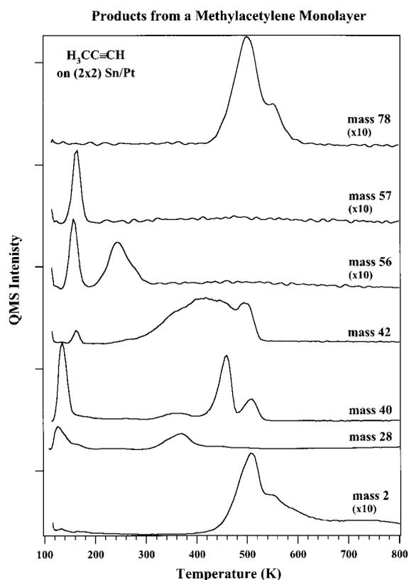
Fig. 7. TPD spectra of products from the reaction of methylacetylene after the adsorption of a coverage slightly greater than 1 ML of methylacetylene dosed at 108 K on the  $(2 \times 2)$ Pt–Sn surface alloy.
