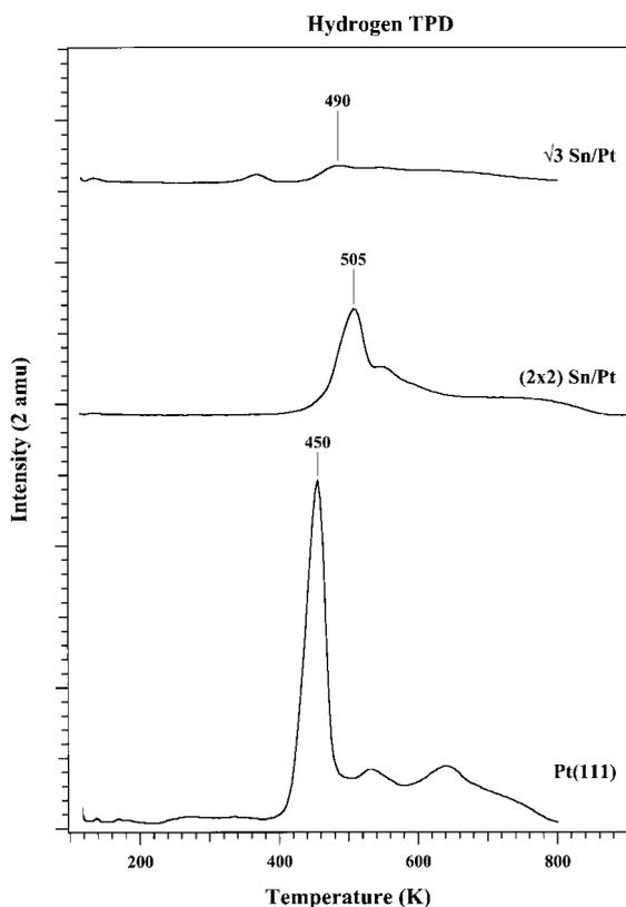
Fig. 5.  $H_2$  TPD spectra after a methylacetylene saturation exposure on the Pt(111),  $(2 \times 2)$  and  $\sqrt{3}$  Sn/Pt(111) surface alloys at 108 K.
