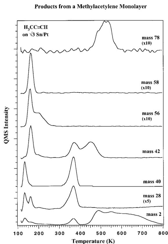
Fig. 8. TPD spectra of products from the reaction of methylacetylene after the adsorption of a coverage slightly greater than 1 ML of methylacetylene dosed at 108 K on the  $\sqrt{3}$  Pt–Sn surface alloy.
