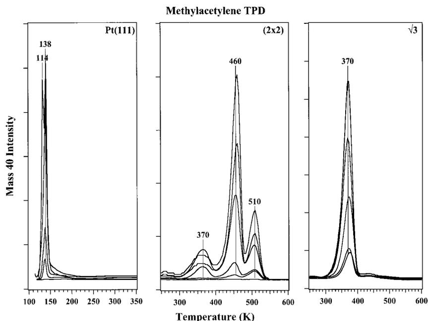
Fig. 2. Methyacetylene TPD for a series of coverages on the Pt(111),  $(2 \times 2)$  and  $\sqrt{3}$  Sn/Pt(111) surface alloys at 108 K.
