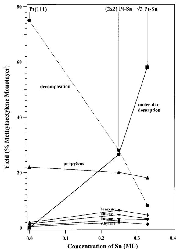
Fig. 12. A quantitative comparison of the relative yields of the major products on the Pt(111),  $(2 \times 2)$  and  $\sqrt{3}$  Sn/Pt(111) surface alloys at saturation coverages.
