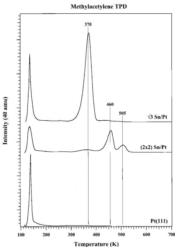
Fig. 3. Methyacetylene TPD spectra after a methyacetylene saturation exposure on the Pt(111),  $(2 \times 2)$  and  $\sqrt{3}$  Sn/Pt(111) surface alloys at 108 K.
