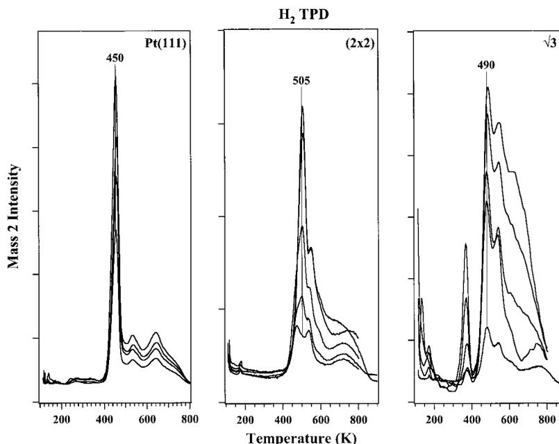
Fig. 4.  $H_2$  TPD for a series of coverages on the Pt(111),  $(2 \times 2)$  and  $\sqrt{3}$  Sn/Pt(111) surface alloys at 108 K.
