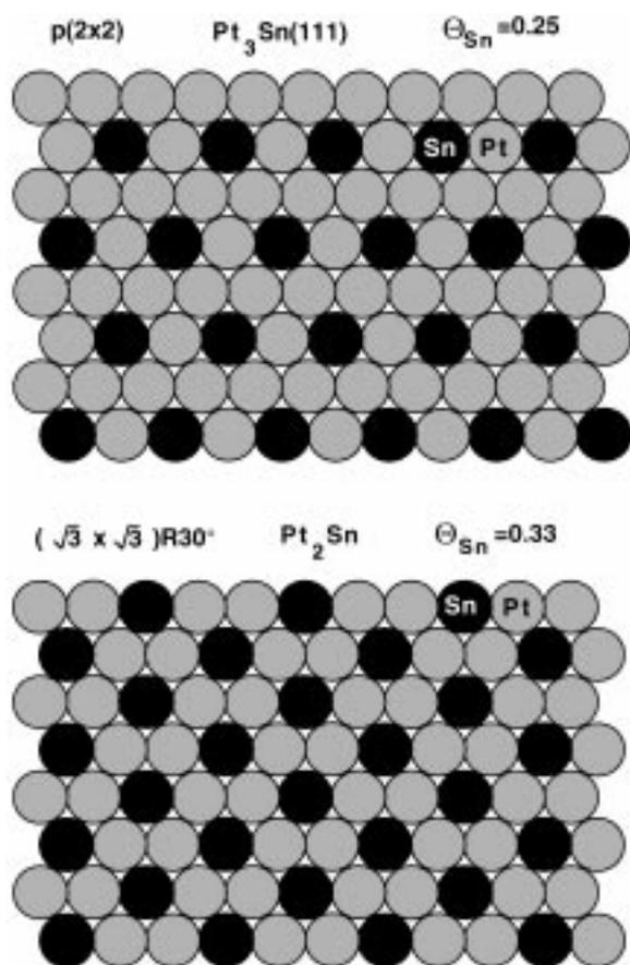
Fig. 1. Schematic top view of the structure of two Sn/Pt(111) surface alloys.
