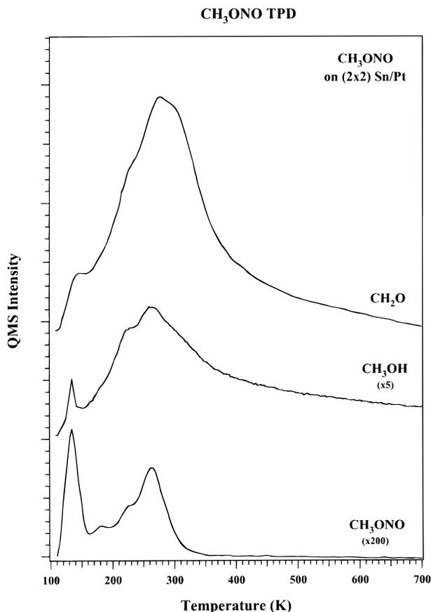
**Figure 1.** TPD spectra of several products following the adsorption of methyl nitrite ( $\text{CH}_3\text{ONO}$ ) on the  $(2 \times 2)$  Sn/Pt(111) surface alloy at 100 K for an exposure slightly larger than monolayer coverage.
